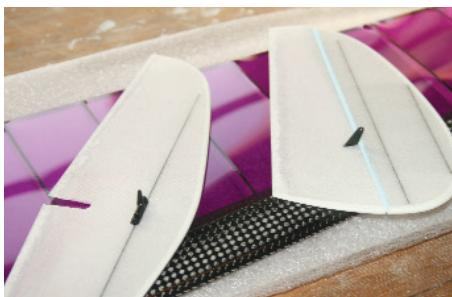
Horns mounted with thin CA which should be sparingly applied to avoid spoiling that beautiful finish!
