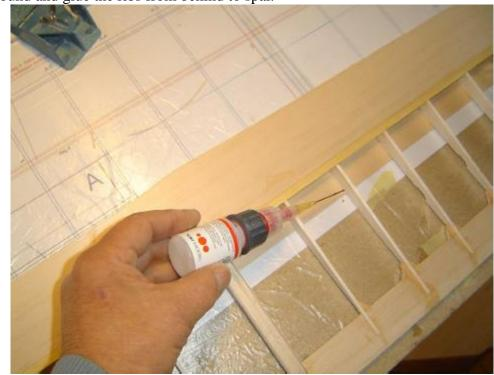
Then turn around and glue the ribs from behind to spar.
