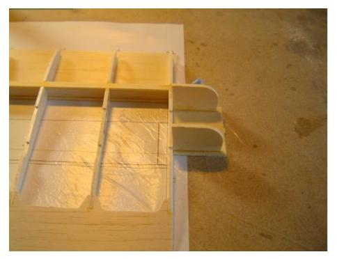
Roughen and thoroughly clean aluminum wing joiner tubes. Slide aluminum tube into ribs A-9 and A-8. Align at 90  $^{\circ}$  to end rib. Gap between tube and spar webbing will be filled in with scrap 1.5mm plywood. Coat ply filler, Al tube, and spar webbing with epoxy and assemble. Picture shows top spar in place, but do this step before top spar is glued in so the ply filler can be inserted.
