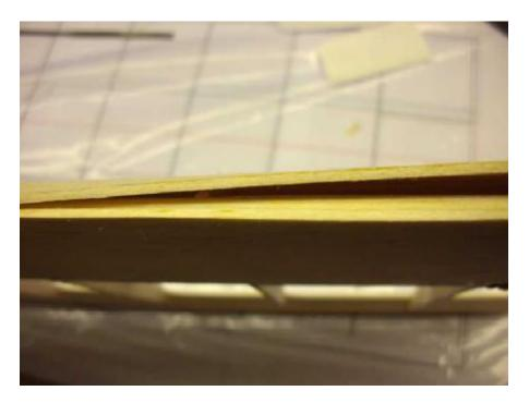
The nose can now be sanded flat from the beginning to the 2 mm bar and a 4x10mm balsa strip leading edge is glued on. Now the middle 1.5mm planking is glued on. Sand the leading edge to shape using the ply jigs to get the correct shape. Each jig has the corresponding rib location on it.
