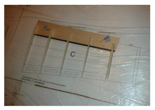
Fit the spar webbing and ribs. Angle rib C1 for dihedral using the 6 degree ply template. Washout can be built into the wing tip, or it can be done with the covering. Glue ribs, spar webbing and bottom spar together. There is no spar webbing between the first two sets of ribs. A plywood angle part is put in here later.
