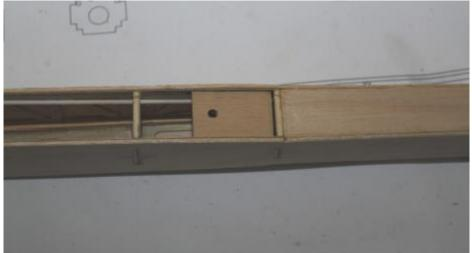
Now the pushrod housings can be glued to the fuse bulkheads.
