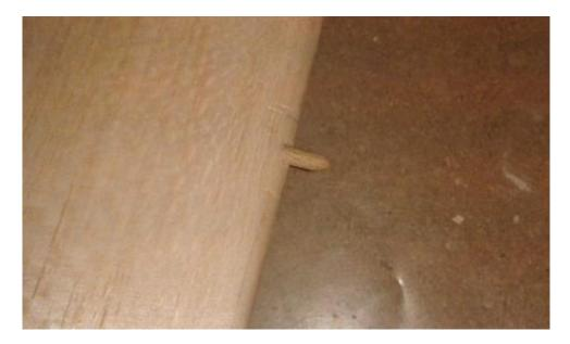
When wing is lined up, glue the ply wing locating piece in the fuselage. Remove the wing and reinforce glue the wing retaining piece in the fuselage.
