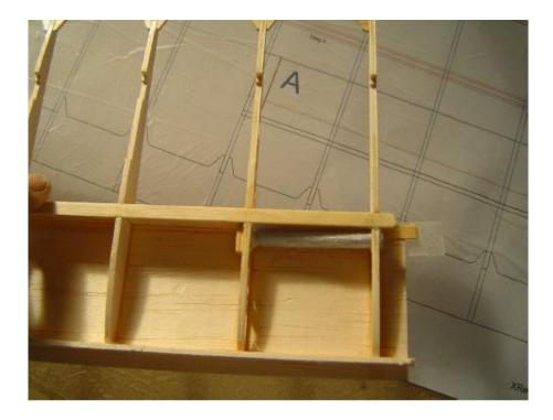
Now the upper planking can be glued to the ribs.
