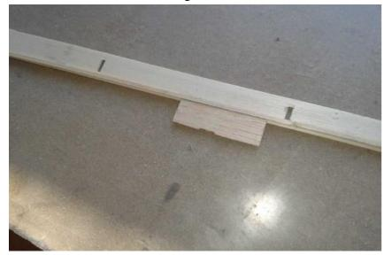
The taper the longerons at the rudder cutout so the back end of the fuse can be glued to the rudder.
