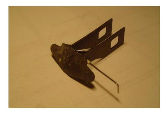
The elevator pivot is located in front of the last bulkhead. Notch the fuse sides for the elevator mounting side plates. Install the horizontal elevator plate onto the side plates using a piece of wire.
