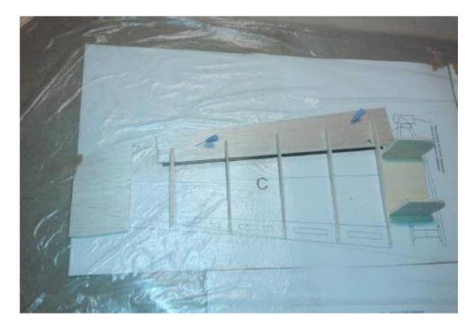
Make a false leading edge from 2mm scrap balsa. Shape top edge for upper planking. Cut top planking so it will extend over the wing tip. Glue on upper planking.
