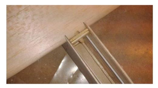
The wing retaining piece in the fuselage.
