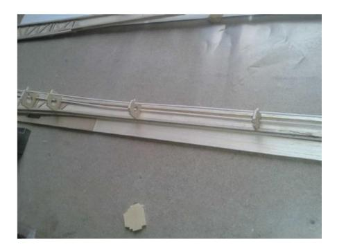
Next, the fuselage sides are glued together. Make sure they are parallel.
