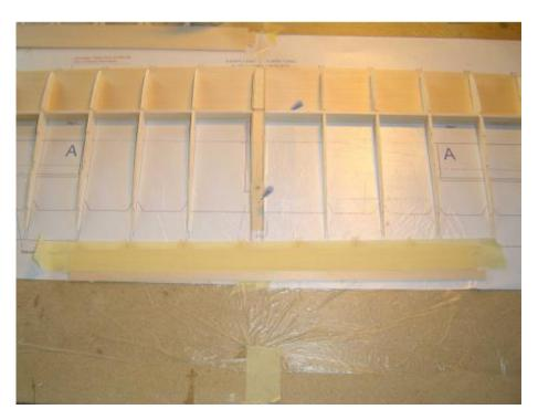
The wing can be turned right side up and the trailing edge can be sanded to a taper on the top side, starting from about 12 mm from the edge, so it is about 1mm thick at the trailing edge. Masking tape can be used to protect the area that is not sanded.
