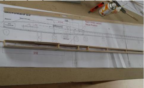
Before the frame is bonded at the end of the plywood reinforcement, insert the wing retainer. Insert the 4 mm sheet of plywood with the 5 mm threaded hole toward the front of the fuselage. Do not glue yet. That is glued later on, when the wing adjustment is made with the locking pin
