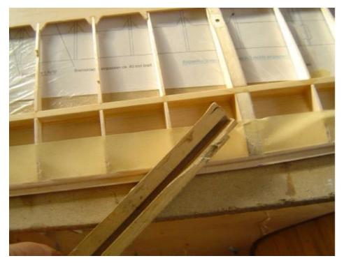
After drying, cover the ribs to protect them and sand the 2mm strip to shape for planking.
