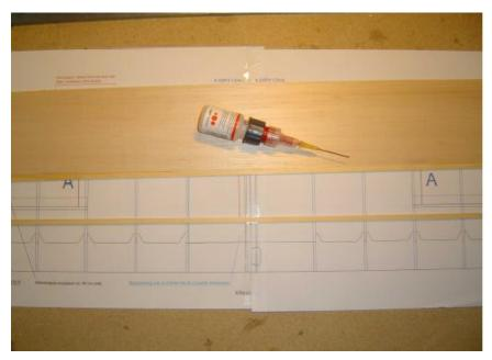
The ribs are cut and sanded to fit on the pine spar. The 3mm balsa spar webbing is also prepared. The two ribs adjacent to the root rib have a section for the webbing.
