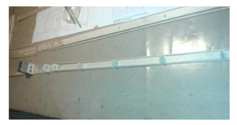
Use a spacer with 2 mm offset to locate the longerons.
