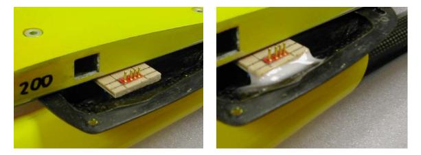
Trimming of the boom/ballast tube is optional if you require additional room for your receiver. Rough cut with a rotary tool grinder, and then smooth with an emery board or sandpaper on a popsicle stick.
