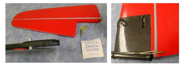
Use a rotary tool to grind out the shear webbing for control rod clearance. (Note that the supplied rods may be too short for the flaps). Solder the clevises to the rods on the servo end. The flap rods also required a bend in order to get full travel without binding. It was also necessary to extend the length of the brass control horn for the flaps by leaving a few threads exposed.
