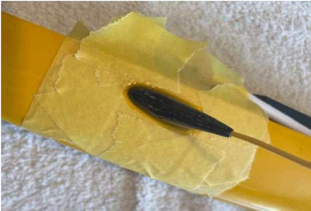
*Aerial fairings in place. Masking tape prevents epoxy going where its not wanted*
