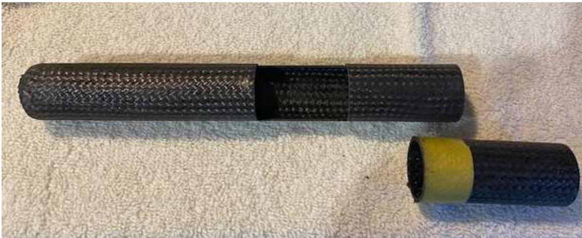
*Mark out and trim the ballast tube to ~160mm*
