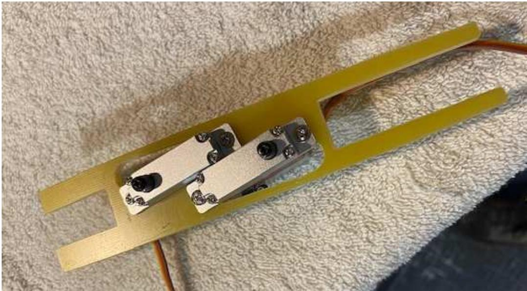
*Servo tray with servos. Remove servos before fitting*
