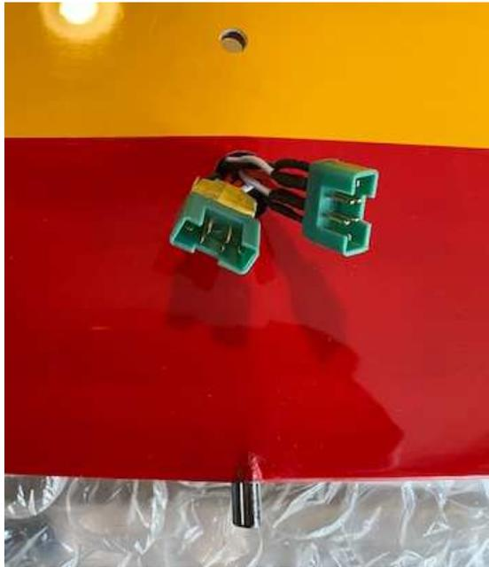
*Wing Harness exit – hole must be enlarged*
