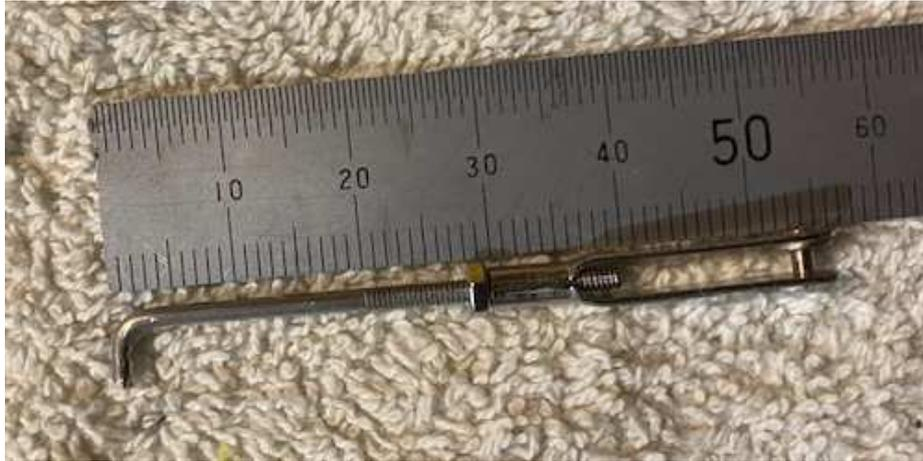
*Set control rod to 53mm long before installation*
