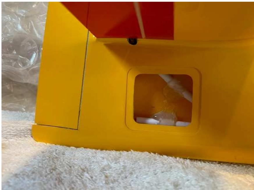
*Snakes held with hot-glue where they touch. Voltage regulator fits forward of the hatch with extended wires to battery and RX*
