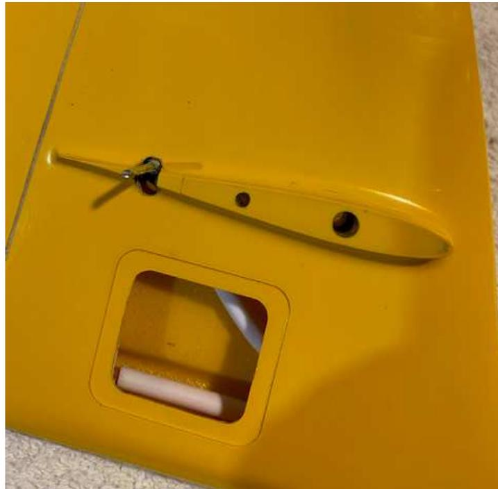
*Elevator slot with Rudder and Elevator snakes in position*
