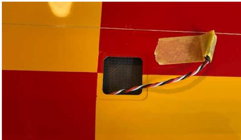
*Retain servo connectors with tape to protect wing*
