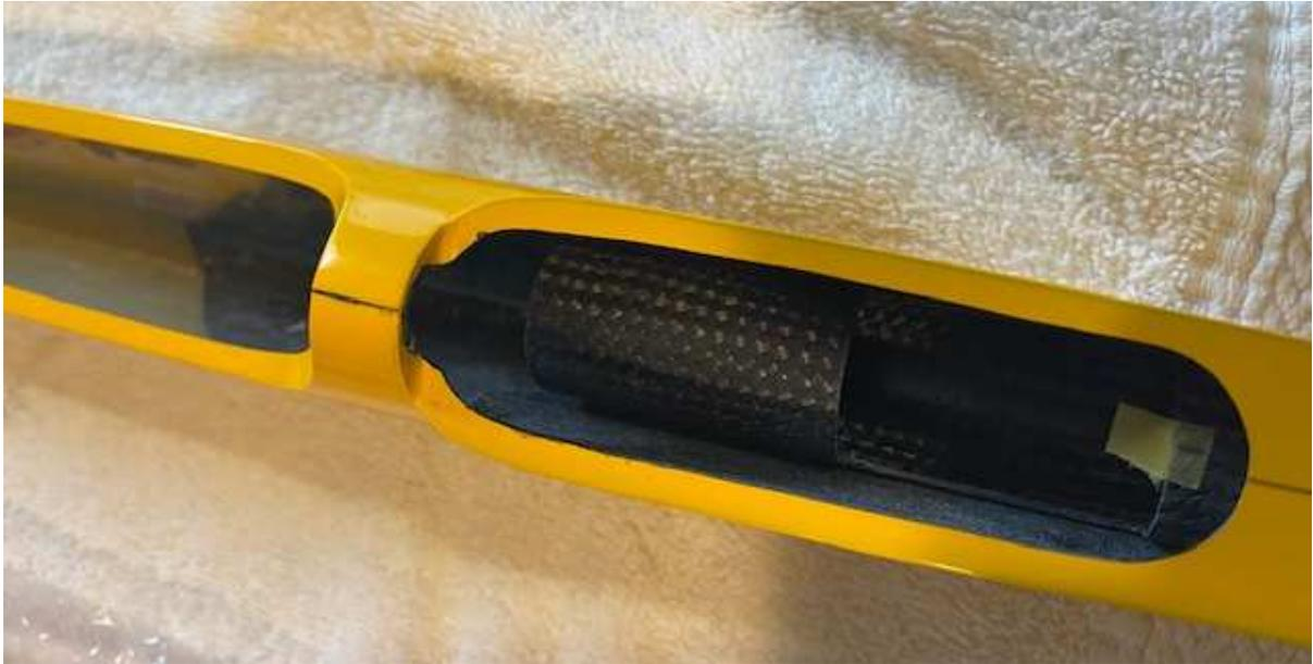
*Ballast tube in place. Note the centre of the tube is aligned to 80mm from Wing Leading Edge*
