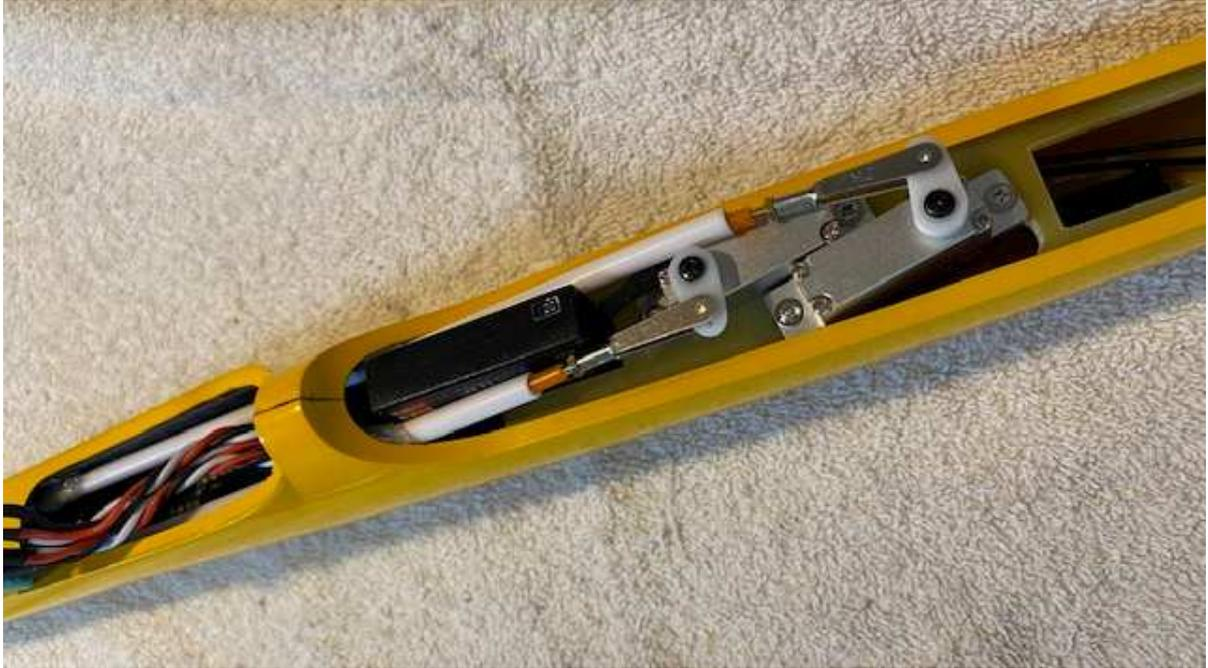
*Servos installed and connected with RX in place*
