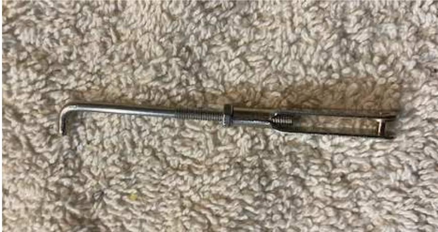
*2mm diameter control rod with metal clevis and lock-nut*
