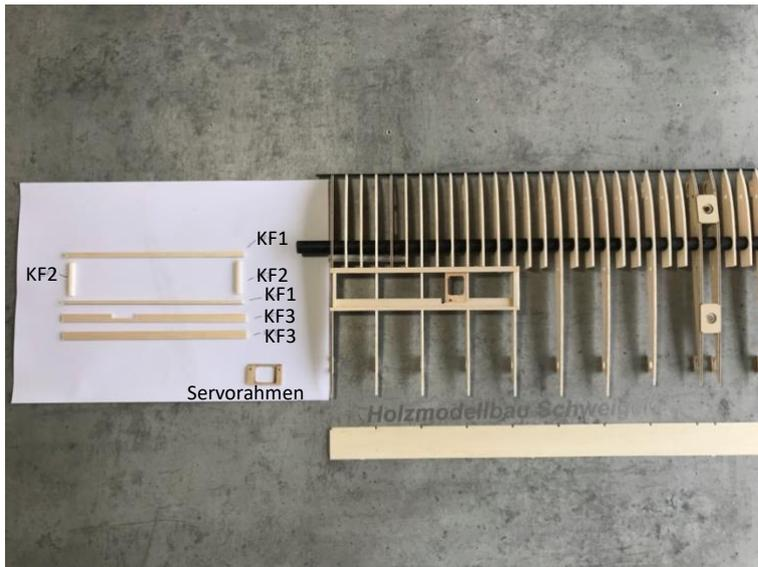
The next step is that Border for the flaps in the area. It will be the parts KF1-KF2 from the 3mm, and the both strips KF3 from the 2mm balsa board required. KF3 is on the balsa board of the ribs (Part A). To note is here that there are two from KF3 different designs gives: once with the cutout for a servo frame and once without the cutout. The Parts are in the area in the meant for
