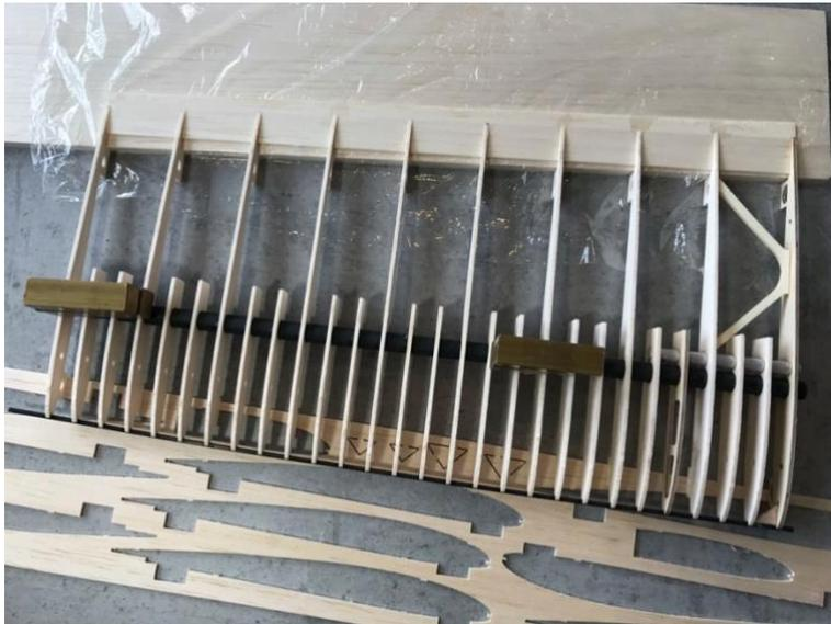
Be careful here: the leading edge in Part A and B are 2.5 mm thick. (In contrast to Part C: here they are only 2mm thick). The wing part B is also again on the leading edge 2mm (under the feet of the Ribs) and on the trailing edge with 8mm underlaid. Thus can the trailing edge free of distortion be glued on. At the end will still be the great reinforcement between the rib B1 and B4 glued in.
