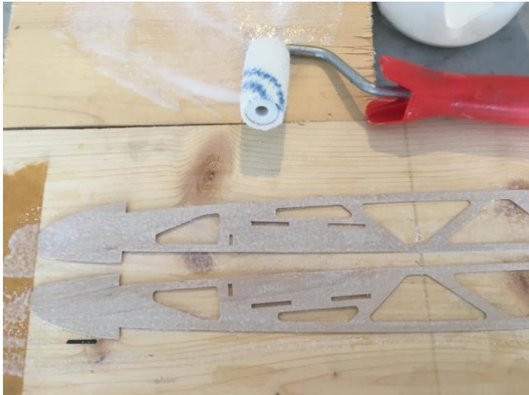
As shown in Fig. 3, we use a roller for gluing R9 and R10. This allows the glue to be applied in an evenly thin layer. Press the parts together for several hours.
