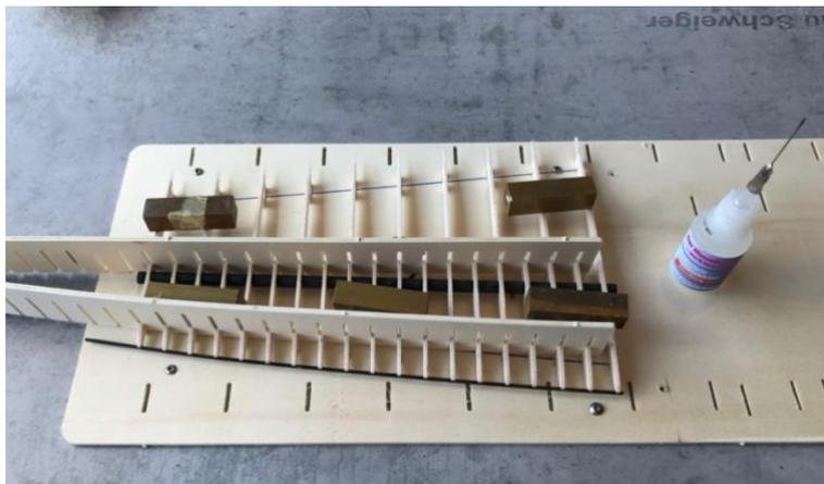
In the end we still check once the correct alignment all ribs and glue all together whole ribs (not the Half ribs) with the pipe. Tip:for correct alignment we use weights to fix the wing part neatly.
