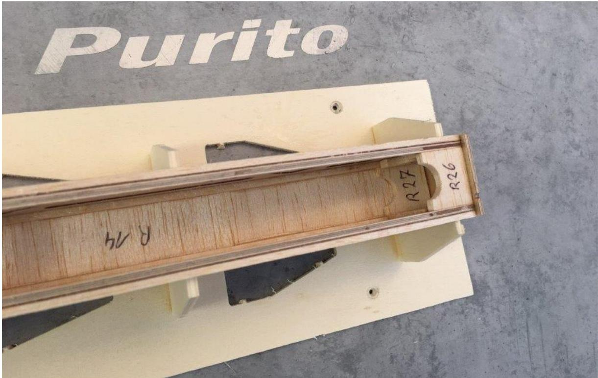
Now parts R25 are glued to both sides of the fuselage, part R26 should be glued to the bottom of the fuselage and part R27 to the top of the fuselage, centered between the two parts R25 (see picture). The parts R25-R27 are there to fit the fuselage to the spinner later.
