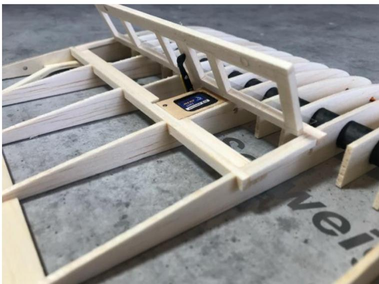
Should our solution be for the Flap opening used will become one Servo arm extension required. Recommend for the servo arms we our GFK extension, together with the matching servo frame as Accessories are available. For the functional ice we have also a video
