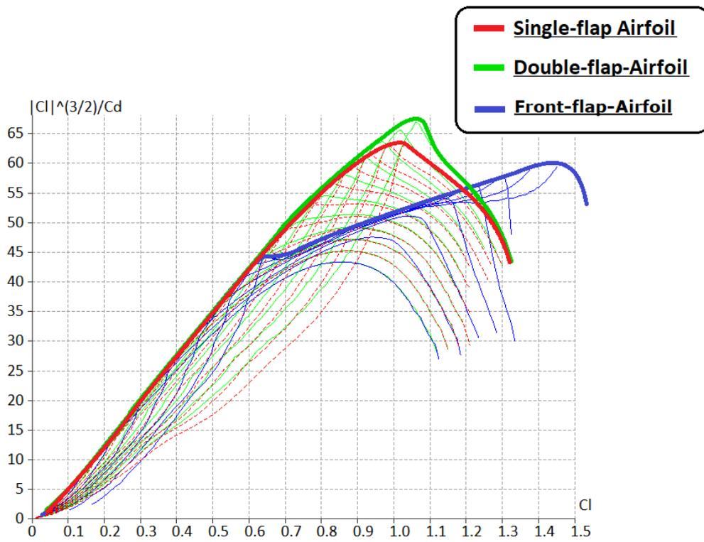
Fig. 21: plot of airfoil endurance parameters for single-flap and double-flap and front-flap airfoils.
