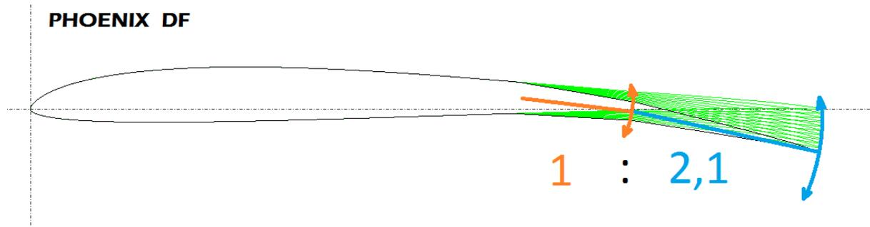
*Fig. 16: optimized coupling ratio between forward and rearward flap*
