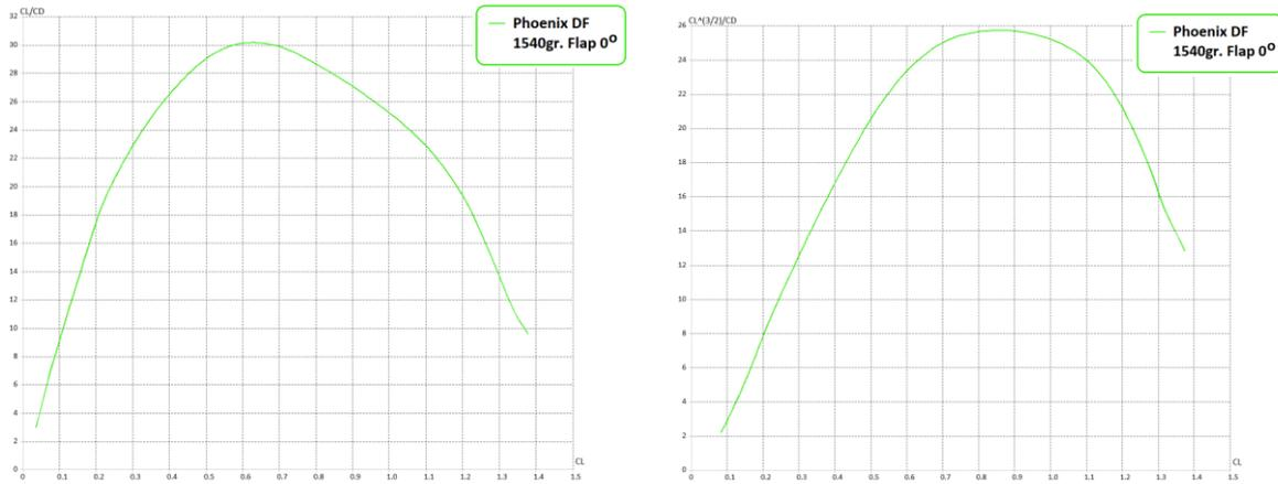
*Fig. 03: Glide ratio and Endurance-parameters over CL*
