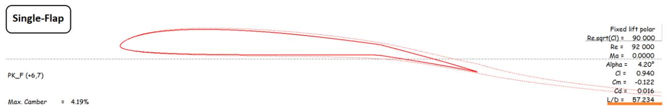
Fig. 09: Boundary layer on single-flap airfoil at  $Cl = 0.94$  and  $Re \cdot \sqrt{Cl} = 90000$
