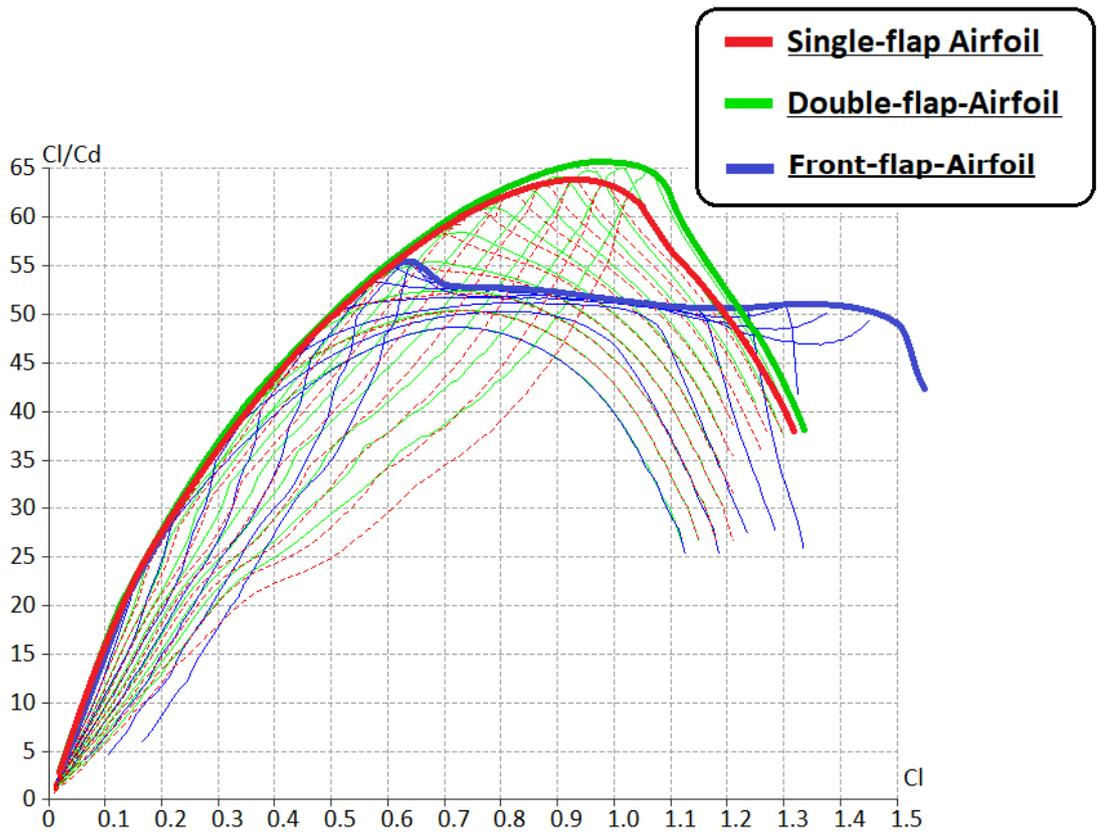
Fig. 20: plot of airfoil glide ratios for single-flap and double-flap and front-flap airfoils.
