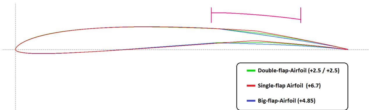
Fig.08: Overlay of the airfoils geometries
