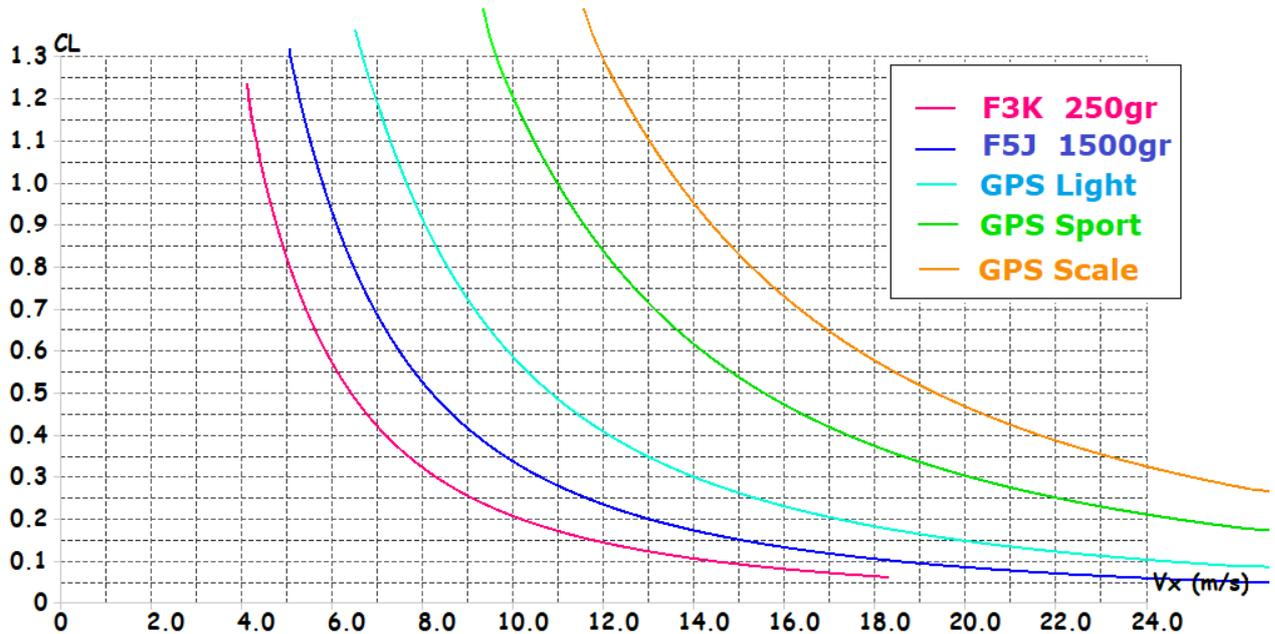
*Fig. 01: relationship between CL and Airspeed for straight line flight.*
