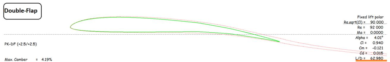
Fig. 11: Boundary layer on double-flap airfoil at  $Cl = 0.94$  and  $Re \cdot \sqrt{Cl} = 90000$
