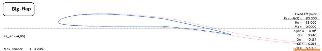
Fig. 10: Boundary layer on big-flap airfoil at  $Cl = 0.94$  and  $Re \cdot \sqrt{Cl} = 90000$
