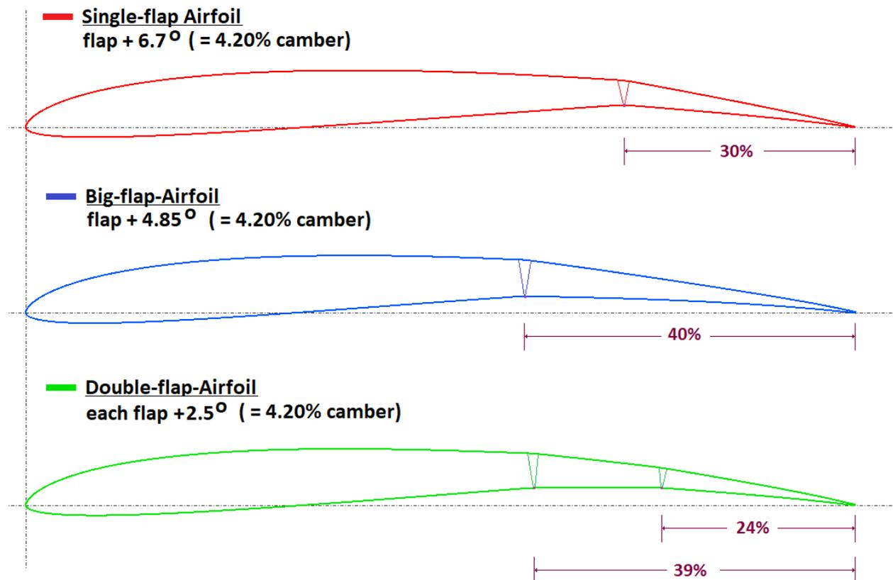
*Fig. 05: Common flap arrangements for F5J models and the "double-flap-solution".*
