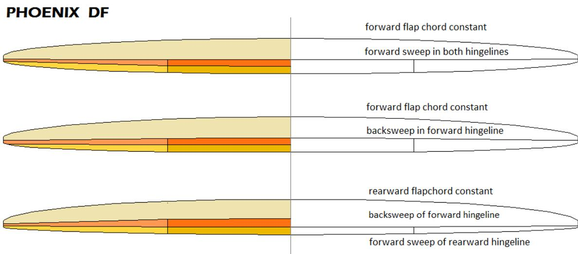
*Fig. 17: development of an efficient wing planform for incorporating the double-flap*
