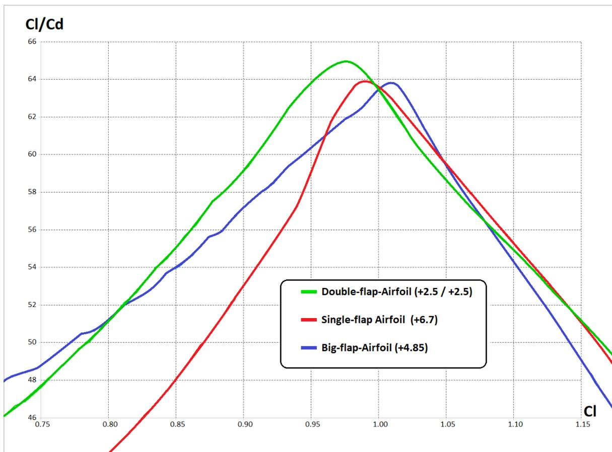
Fig. 06: LD-values of the examined airfoils in a  $Cl$ -range between 0.75 and 1.15
