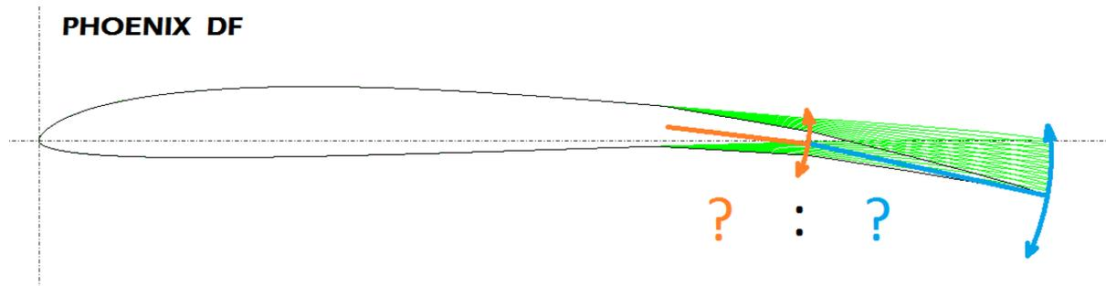
*Fig. 15: finding the right mixing ratio between forward and rearward flap deflection*
