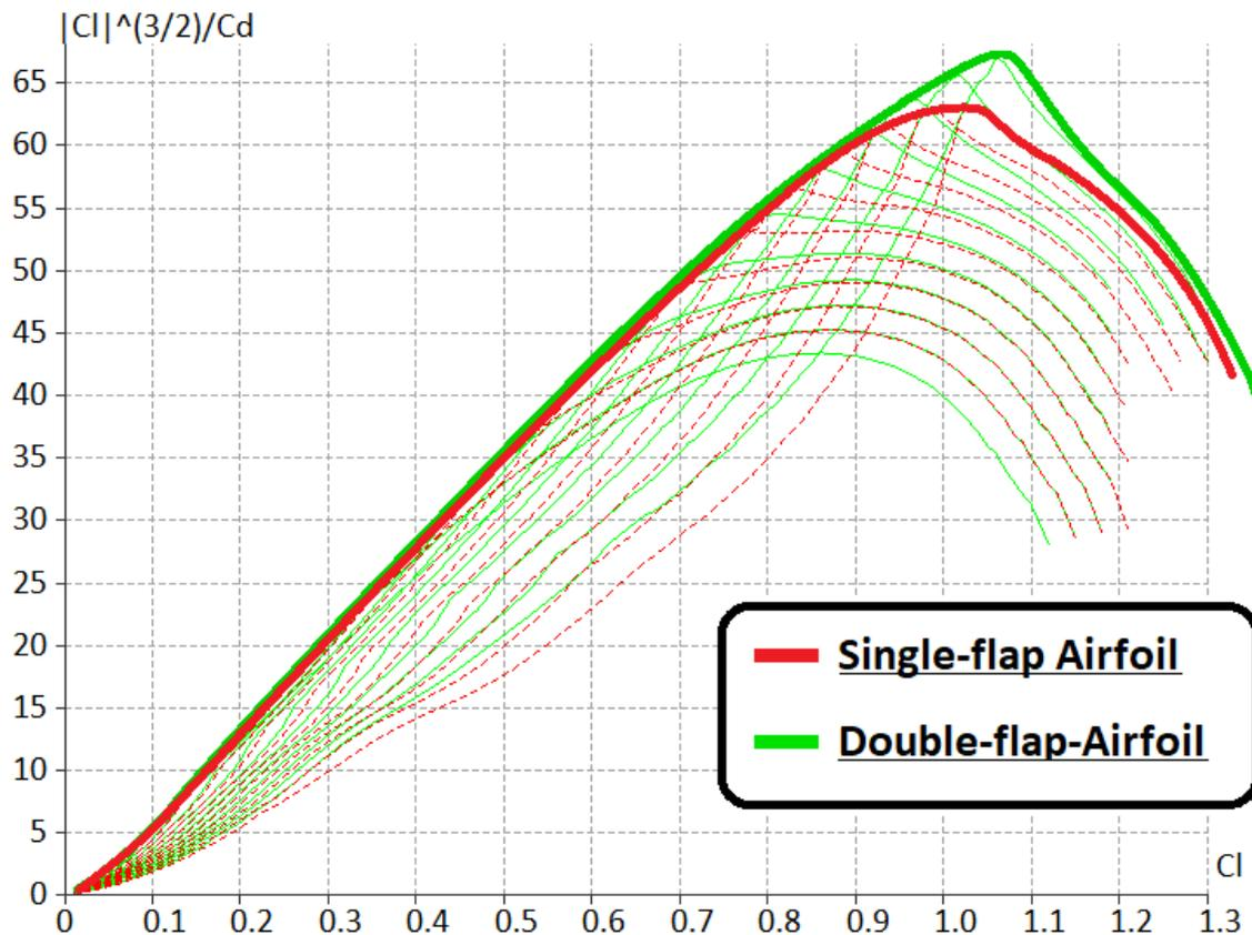
*Fig. 14: plot of airfoil endurance parameters for single-flap and double-flap airfoil over lift coefficients for various flap angles.*
