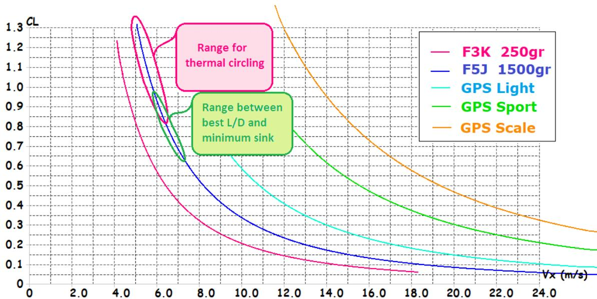
*Fig. 02: operating range for 90% of an F5J models flight envelope.*
