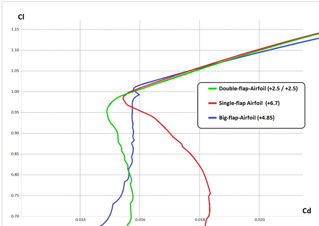
Fig. 07: Cl/Cd Diagram with respective polars for the observed airfoils
