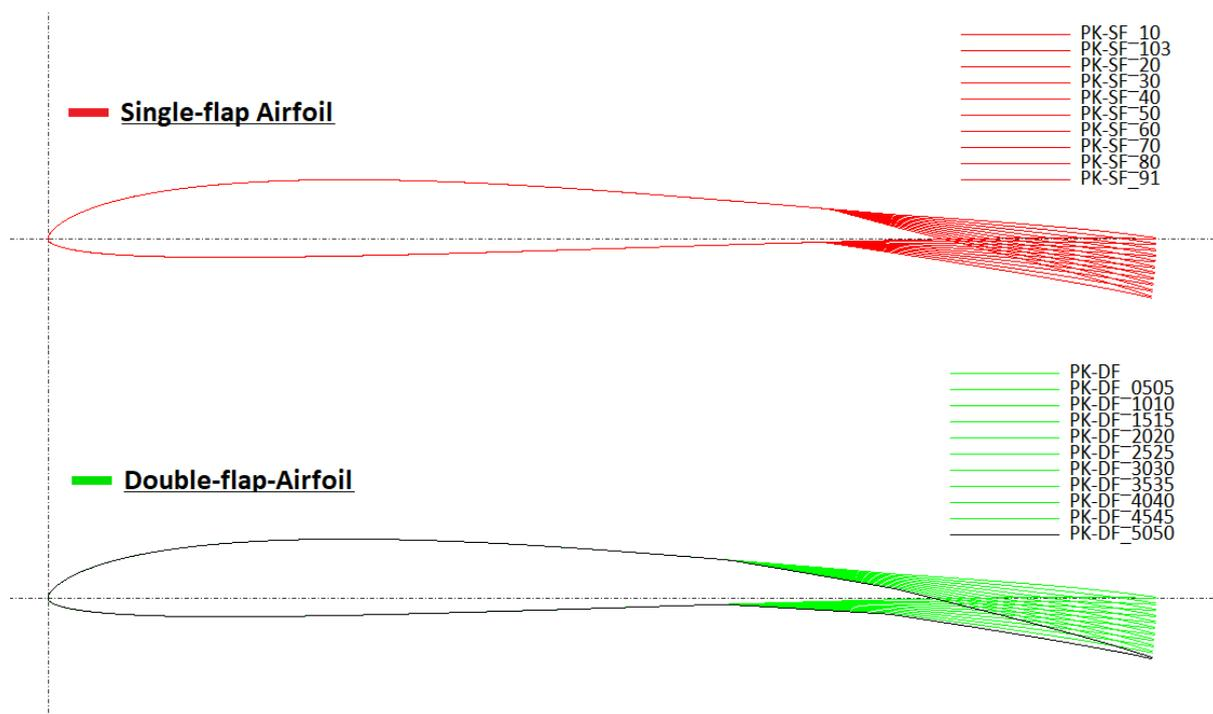
*Fig. 12: Comparison of flap angle envelopes*
