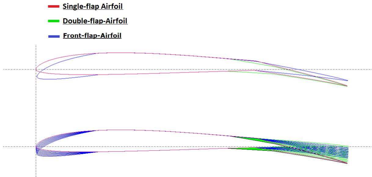
*Fig. 19: comparison of double-flap and front-flap airfoil*
