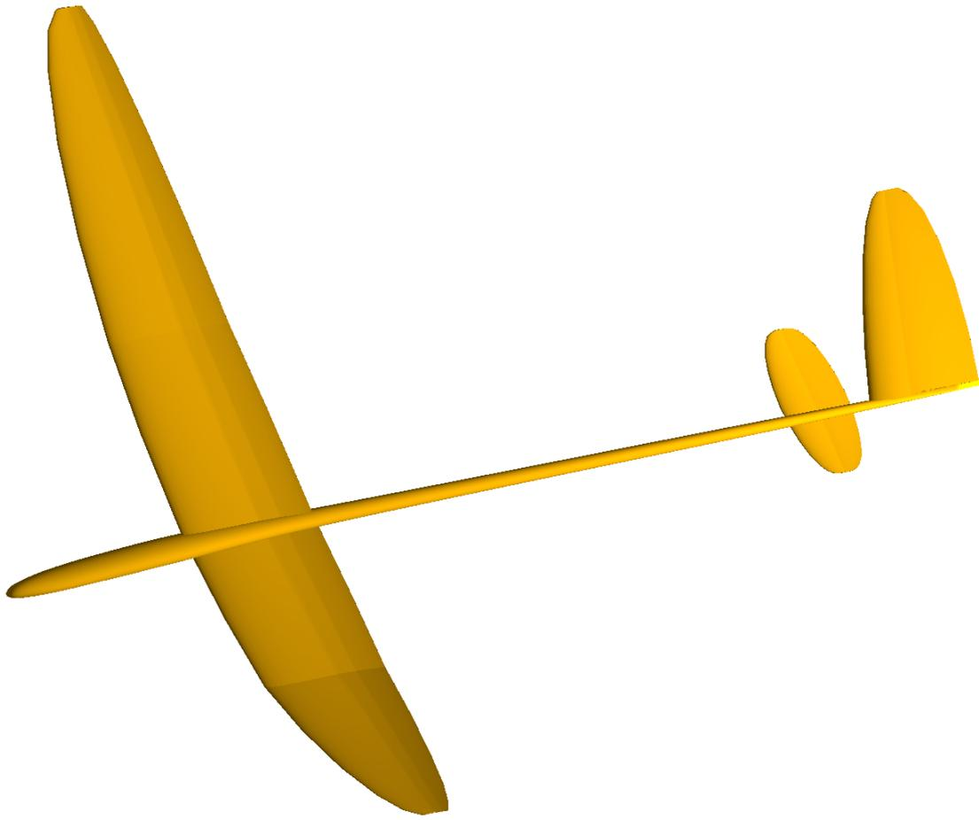
*Fig. 22: The PHOENIX DF with visible hinge lines on the double-flap wing.*
