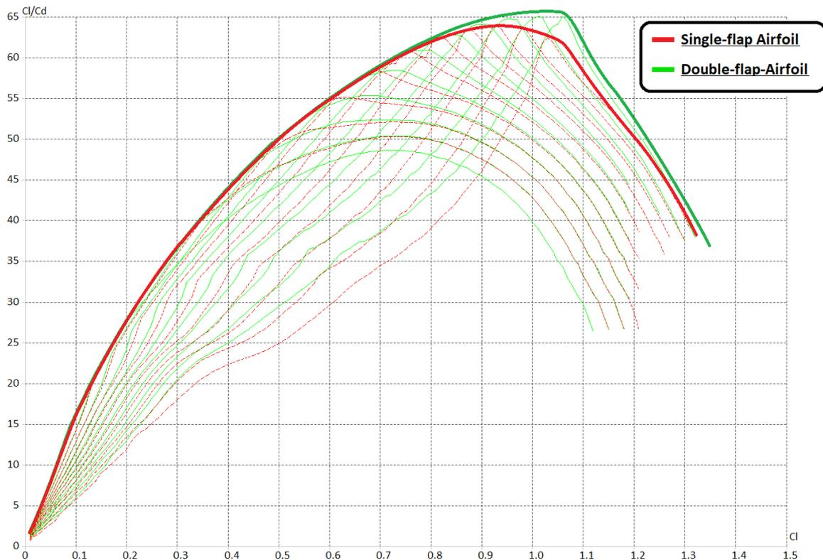
*Fig. 13: plot of airfoil glide ratios for single-flap and double-flap airfoil over lift coefficients for various flap angles.*
