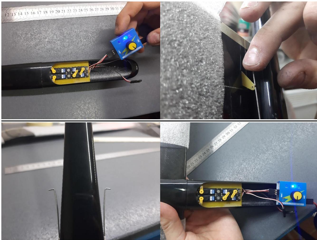
Lay rods through fuselage, put tubes 5mm length on rods and glue them between two servos.
