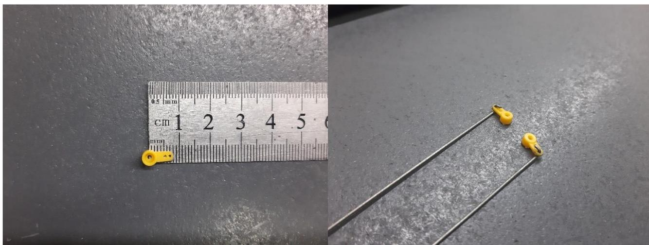
Set aileron servos horns 30-40 degrees back at neutral servos position.
