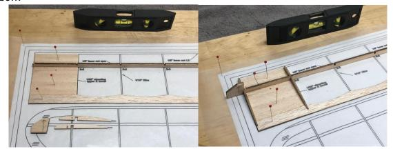
4. Add the 4 R-3's and 1 R-4 ribs and glue in place.
