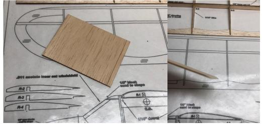
7. Trim the forward edge of the sheeting until the tapered part is even with the trailing edge and glue in place.
