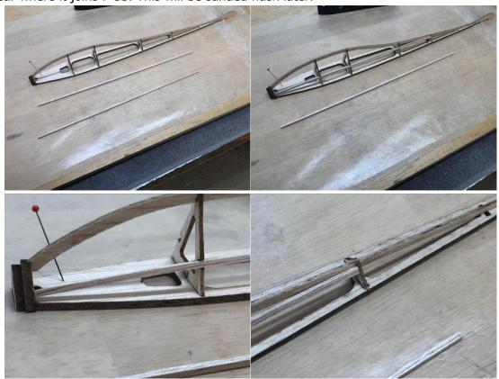
6. Locate and glue the 2 nose doublers in place flush to the rear of N-1
