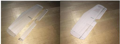
• If the elevator hinge is too tight, you can head it it up with your iron and flex it further if necessary.
