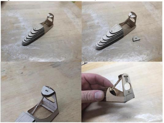
19. Fuselage construction is now complete. You can now sand the nose to shape, and all stringers flush.
