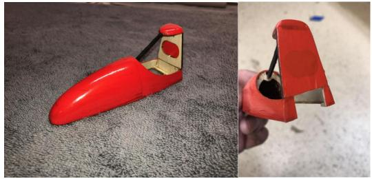
• I covered the fuselage in 4 pieces, splitting it in upper and lower as well as left and right sections. I started with the lower left and covered up to the crutch, then right up to the crutch.
