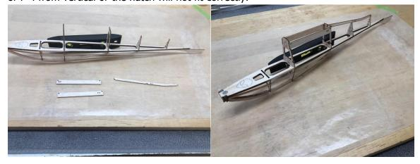
9. Locate the two shorter 3/32 stringer pieces. These will fill in the area behind the wing saddles back the spine and F-5. These will also be trimmed to fit, glue in place.
