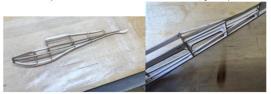
10. Locate the 1/32" tail saddle pieces. Glue these one at a time to the crutch and F-6. Again make sure that these are square and vertical. A small gap remains at the top front area for the fin to slide between.
