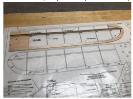
3. Locate the dihedral gauge, R-1 and R-2. Using the gauge, place R-1 at the proper angle on the spar with the notch tight at the trailing edge. Add R-2 the same way, but vertical. Glue both ribs in place along with the spar to the bottom sheeting, trailing edge and tip bow.
