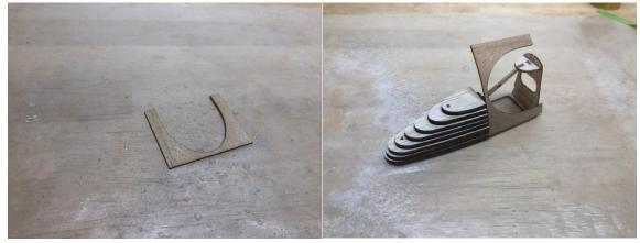
18. Bend it the rest of the way around and glue it to the other side. Trim the ends of the sheeting flush with the back of H-3. Glue H-5 on top of H-5.
