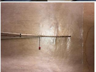
5. Locate 2 of the 3/32" stringers. These are taped to the inside of your kit box along with the pushrods. These will need to be trimmed to the proper length before being glued in place. Note that the front bends to meet the rear of N-1, and also sits a bit proud at the rear where it joins F-5b. This will be sanded flush later.
