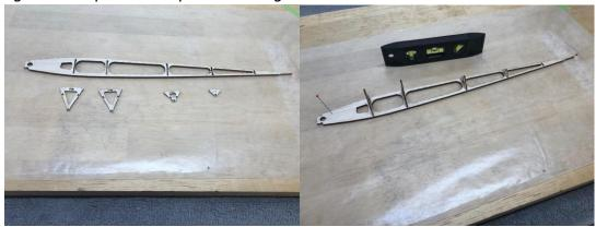
2. Locate one of the magnets. Press it fully into the hole until it is flush against the board and glue in place with medium CA.
