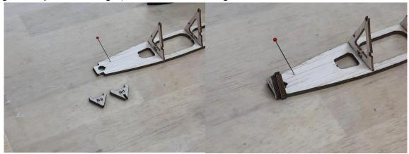
4. Locate the bottom spine and dry fit it into place. Do not glue this until it is fitting flush will all of the formers. It fits nicely so don't force it. Pay special attention at the rear of the fuselage to keep it straight and vertical. This forms the bottom of the fin/rudder assembly and also functions as the tail skid, any misalignment will be visible while flying.
