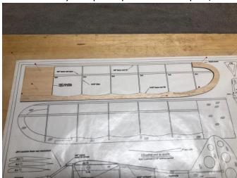
2. Locate the 1/8 spar and position it in place over the plan, but do not pin.
