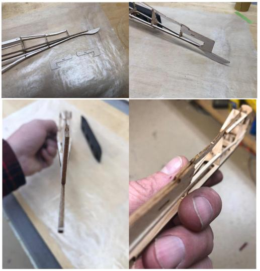
11. Fit the remaining two 3/32" stringers from the tail saddle all the way forward to F-3. When fit correctly, the stringers will be slightly proud of the tail saddles, these will be sanded flush later. Trim them flush with the front of F-3.
