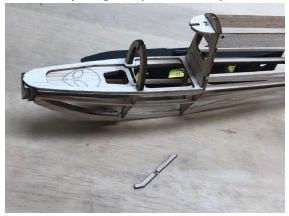
15. Carefully remove the hatch from the fuselage and locate the 1/8" hatch nose blocks numbered 1-8. Glue them to H-1 and H-2 in order starting with #1. Try to only glue around the inside edge of the wood, this will make sanding later much easier.
