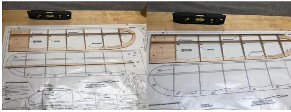
6. Find the 1/32" top sheeting with the etch mark. Taper the sheeting to a point from the etch mark to the edge.
