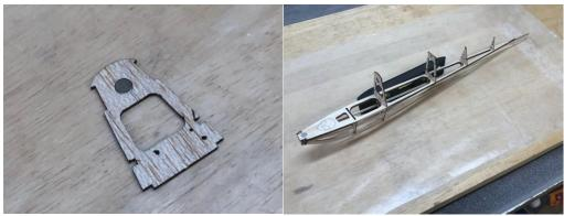
8. Locate the 2 F-7 wing saddles and F-8 upper spine. Glue the saddles in place taking care to get them as even as possible with each other. Care must be taken to not distort F-3 or F-4 from vertical or the hatch will not fit correctly.
