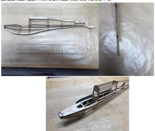
12. Locate H-1 (hatch base), H-3 former and two washers out of the hardware bag. Remove the area inside the etched circle with the tip of an X-acto blade until the washers sit flush with the surface. When satisfied glue in place with Med CA.
