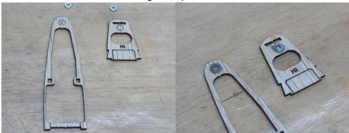
13. Glue H-3 (facing aft) to H-1 keeping it square. Fit H-2 in place (1/8") and glue. Glue H-5 into the slot in H-3, again keeping it square.
