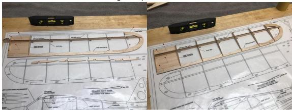
5. Place the 1/8" leading edge up against the ribs and pin in place. The notch in the tip will extend over the tip bow a little and will be sanded flush later.
