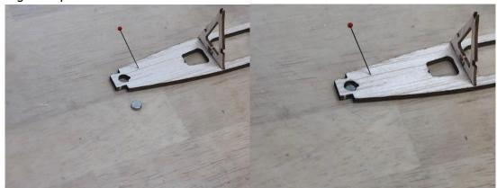
3. Locate the N-1 & N-2 nose blocks. Glue N-1 in place first followed by N-2. Try to keep glue away from the edges, this will make sanding later much easier.
