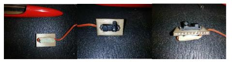
• I used 320 grit sandpaper to roughen up the fuse as well as the milling cutter (by hand), I then cleaned with isopropyl alcohol. Note\* The servo just touches the fuse bottom.
