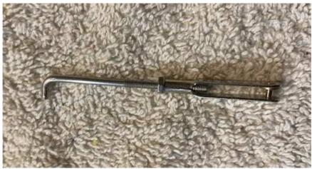
2mm diameter control rod with metal clevis and lock-nut
