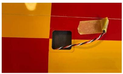
Retain servo connectors with tape to protect wing
