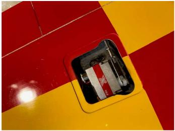
Completed servo installation. Repeat four times
