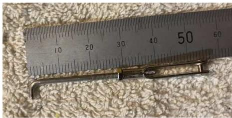
Set control rod to 53mm long before installation
