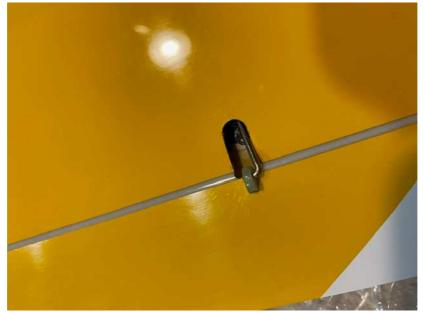
Control horn exit needs to be 12mm long x 6mm wide for smooth operation
