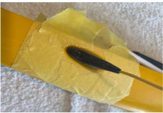
Aerial fairings in place. Masking tape prevents epoxy going where its not wanted
