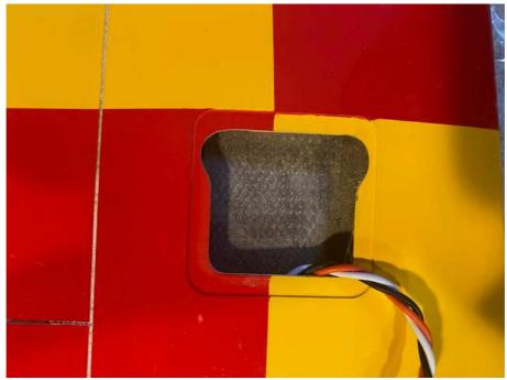
Relieve servo hatch as shown to allow free movement of control rod and output arm. Note that the relief is in-line with the control horn
