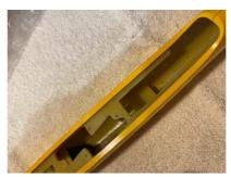
Plates and Servo tray epoxied into the fuselage
