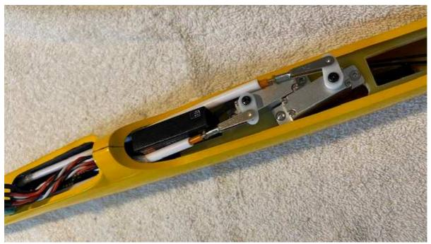
Servos installed and connected with RX in place
