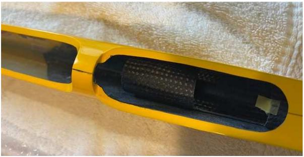
Ballast tube in place. Note the centre of the tube is aligned to 80mm from Wing Leading Edge
