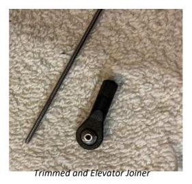
I chose to drive the Rudder and Elevator using 2.9mm snakes with M2 studding each end for the clevises. As the Elevator is top hinged, it is generally less load and easier on the servo to pull at an
