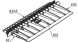
Regrind the tube, leading edge and trailing edge on side ribs.
