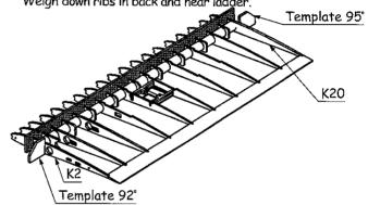
Glue leading edge and wing trailing edge on ribs K2, K12 a K20.
