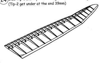
Glue center with tip by epoxide using joiner under 10° angle (end of tip-1 get under 79mm) Gently regrind tubes inside.
