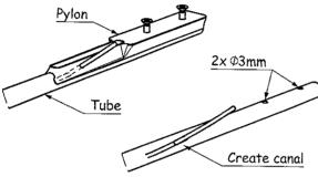
28) Screw the elevator on pylon. Glue the pylon on tube than, controll elevator with wing.
