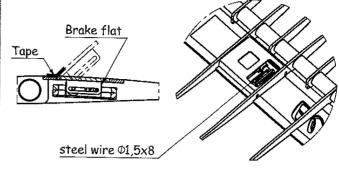
Measure the leghth of tube according to plan, add pylon and mark the place for canal for rod of rud and screws of elevator Ø3mm.
