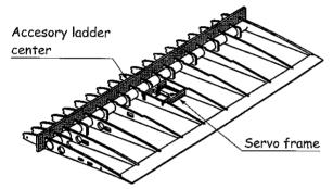
Constitute rib K2 according to plywood template 92° cut B-B
