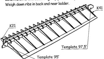
Glue leading edge and trailing edge on ribs K21, K27,K35 and K41. Than glue ribs on trailing edge (thin second glue). Rest ribs will be synchronized on leading edge and can be glued. Glue the tube with middle thin second alu
