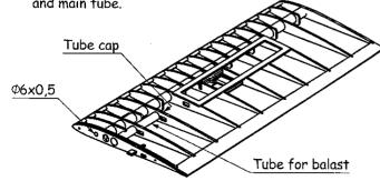
Finish glueing the cover from B.1,5, glue braces B.2 mm Glue the magnet D10x1 and steel wire  $\phi$ 2x12 in
