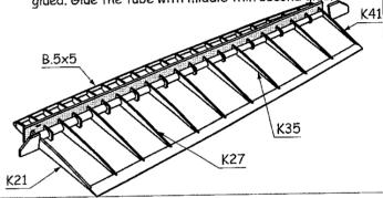
Shave leading edge and trailing edge, regrind to profile. Glue the brace B.2mm
