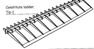
19) Constitute rib K21 according to plywood template 95 cut C-C. Constitute rib K41 according to plywood template 97,5°cut D-D
