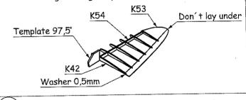
23 Softly regrind the ribs into the form of leading edge. Glue leading edge B.3×7.
