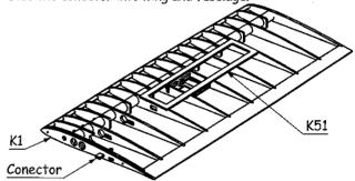
Glue the tubes into ribs and plywood tube cap into tube for balast using epoxide. Create overpass from epoxide between tube  $\phi$ 6x0,5 and main tube.
