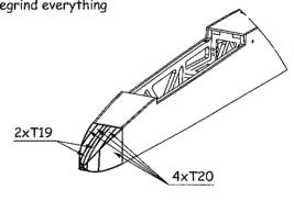
$\widehat{7}$ ) Glue the laminate tube in  $\Phi$ 6x0,5
