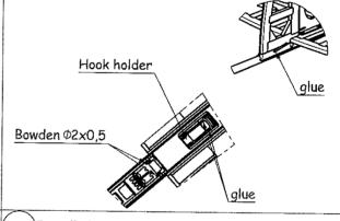
Cover the model, glue flaps and brakes with tape. Controll turning of the wing, on tip-1 negative 1-2mm and on tip-2 negative 2-3 mm. Glue levers on rud and elevator. Use steel wire  $\phi$ 0,8mm as a rod. Curve on the rudder and servos into L or Z shape.
