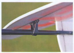
thought within the DLG world that the rudder linkage should be under tension and not compression when the model is launched which, as illustrated, would be the case for a right-handed throw. That said, I can't see how it would make much difference here; everything is so light that the launch forces shouldn't affect it if on the 'wrong' side.
