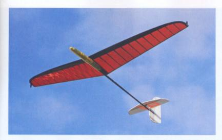
D-box is beautifully curved around the planform of the wing, and at either tip there's a slot for bonding in a supplied launching winglet, making the model suitable for left- or right-handed launchers.
