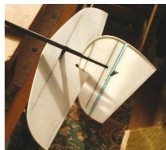
*The translucent tail surfaces are exquisite. Note the clearance slot for the AMT - check alignment before gluing in place!*
