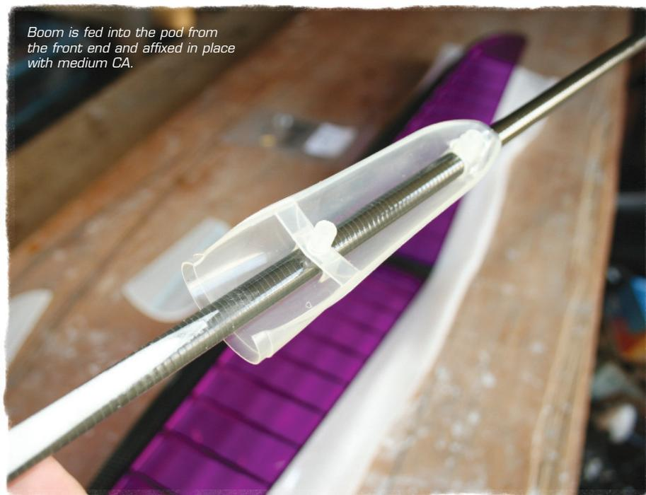
Boom is fed into the pod from the front end and affixed in place with medium CA.
