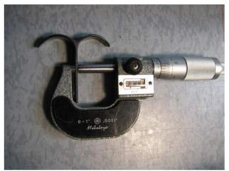
**Step 1**: Measure thickness of blade tongue.
