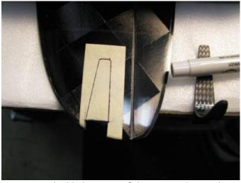
**Step 5**: Lay the blade on top of the wing and trace the tongue outline onto the masking tape.
