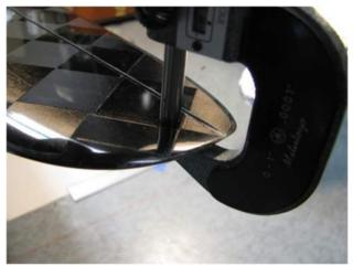
**Step 2**: Measure the thickness of your wing tip to determine the furthest point aft that the tongue will fit within the wing. Remember to add .012" to .016" to the external wing thickness measurement to allow for wing skin thickness.
