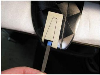
**Step 8**: Use a thin file marked for depth of cut to scrape any remaining foam from the inside face of the wing skins. This ensures the best possible bond between blade tongue and wing skins.
