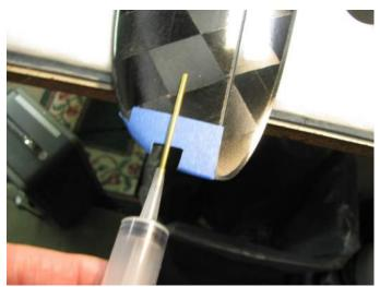
**Step 10**: Use a hypodermic with a large needle or with a 1/16" length of brass tube fitted for injecting the cavity with adhesive.
