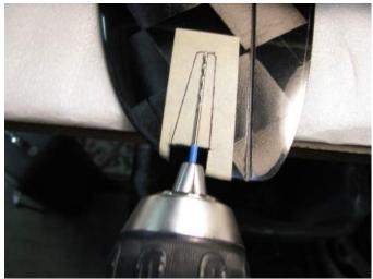
**Step 6**: Mark a 1/16" diameter drill bit for depth of cut by wrapping with masking tape. Use the bit in a drill to remove the foam within the outlined area. Try not to remove foam beyond this area to minimize the amount of adhesive needed to secure the blade in the wing.
