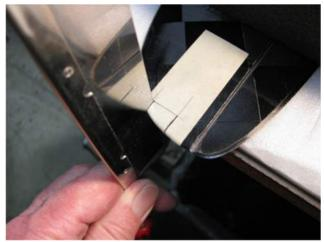
**Step 3**: Lay out to cut a notch for insetting the blade. The aft line should be 3/8" deep and parallel to the hinge line. The notch should match the width of the blade. Use a thin fine-tooth x-acto saw for these cuts. Draw the saw backwards to make the cuts so the teeth don't chip the thin wing skins.
