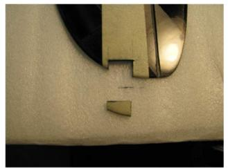
**Step 4**: Use a thin Dremel cut-off disk or a straight Edge and #11 knife blade to make the right-angle end cut. Save the cut-out piece for step #11
