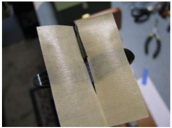
**Step 12**: Mask the center of the blade and sand the area where the in-fill piece will make contact. Remove the tape after sanding.
