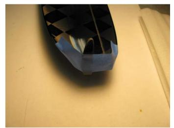
**Step 11**: Slowly insert the blade tongue into the epoxy filled cavity. Wipe off the excess resin as it gets pushed out of the opening.
