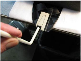
**Step 7**: Use a straw to blow out the loose foam particles and dust as you work through steps #6 and #8. Do not use compressed air as excessive pressure will risk delaminating the wing skins from the core.
