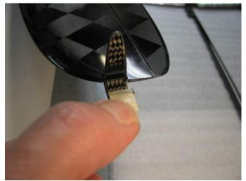
**Step 11**: It is recommended that the wing notch piece be saved and cut-down to fair back into the wing tip. Wrap tape around the piece leaving an excess tab of tape to hold onto.
