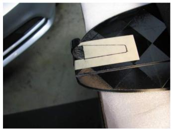
**Step 9**: Dry test fit the blade into the recess to make sure that it seats full depth and without obstruction.
