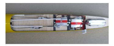
The aileron servos were mounted in the underside of the servo tray:
