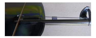
The all moving elevator link was straightforward (well something had to be!). I raised the last guide 0.5mm to help give a smooth run to the horn:
