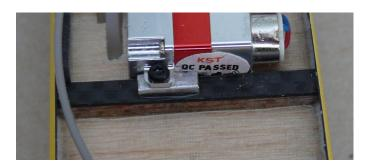
The elevator and rudder servos where mounted on top of the servo tray, behind the battery:
