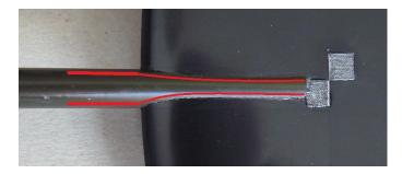
I again used epoxy. I had masked off the rudder around the joint and the outside of the boom before assembly to aid removal of a small amount of surplus adhesive. This also helped giving a minimal sanding of the rudder side of the joint to remove the gel coat and get a better joint.
