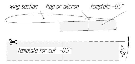
4) Maximum THERMAL flight mode. Also for LANDING mode for ailerons.
