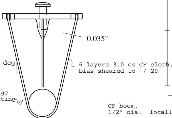
ten 1K CF tows around pin holes in V-strut layup
