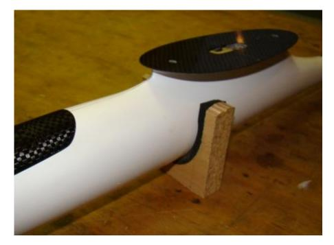
Fig. 10: Rectangular wood fuselage support
