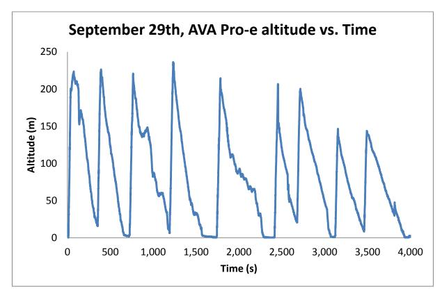
The first observation is that I could fly a quite long time (more than one hour) on a single battery, a 3 elements Li-Po of 2200 mAh capacity. As can be seen, I could climb 9 times out of this single battery. In climb, the motor uses around 25 Amp. so the time to discharge the battery is around 5 minutes, or 300 seconds.
