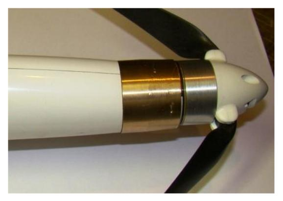
Fig. 6: Propulsion system: the motor is attached in front of the fuselage, rather than installed inside. The brass adaptor is fixed and surrounds the motor. The aluminum adapter rotates with the propeller.
