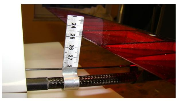
Fig. 11: Small tool to check the elevator settings
