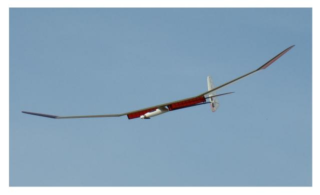
Fig 15: The AVA Pro-e in a steep but slow dive with the flaps down
