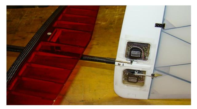
Fig. 4: The rudder and elevator servos are installed in the fixed part of the rudder
