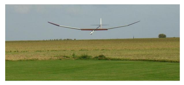
Fig. 15: The AVA approaching landing with the flaps down. It's time to put the flaps back up to avoid damage when the flaps hit the ground
