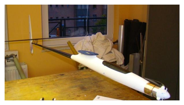
Fig.8: Suspension jig used to balance weights in the fuselage
