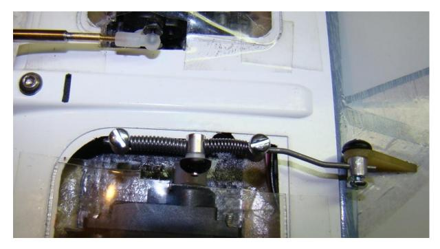
Fig. 5: Rudder servo saver to protect the servo from the shocks in transport.
