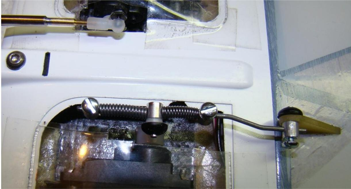
Fig. 5: Rudder servo saver to protect the servo from the shocks in transport.
