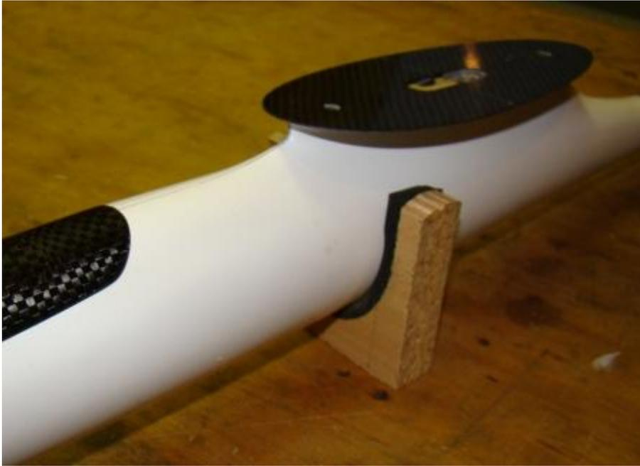
Fig. 10: Rectangular wood fuselage support
