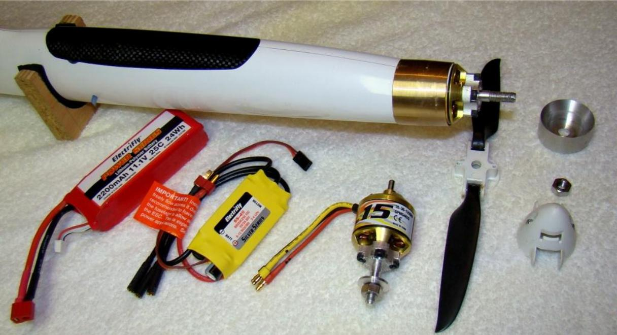
Fig. 7: Propulsion system selected for the AVA Pro-e. A second motor is pictured besides the one already installed on the glider
