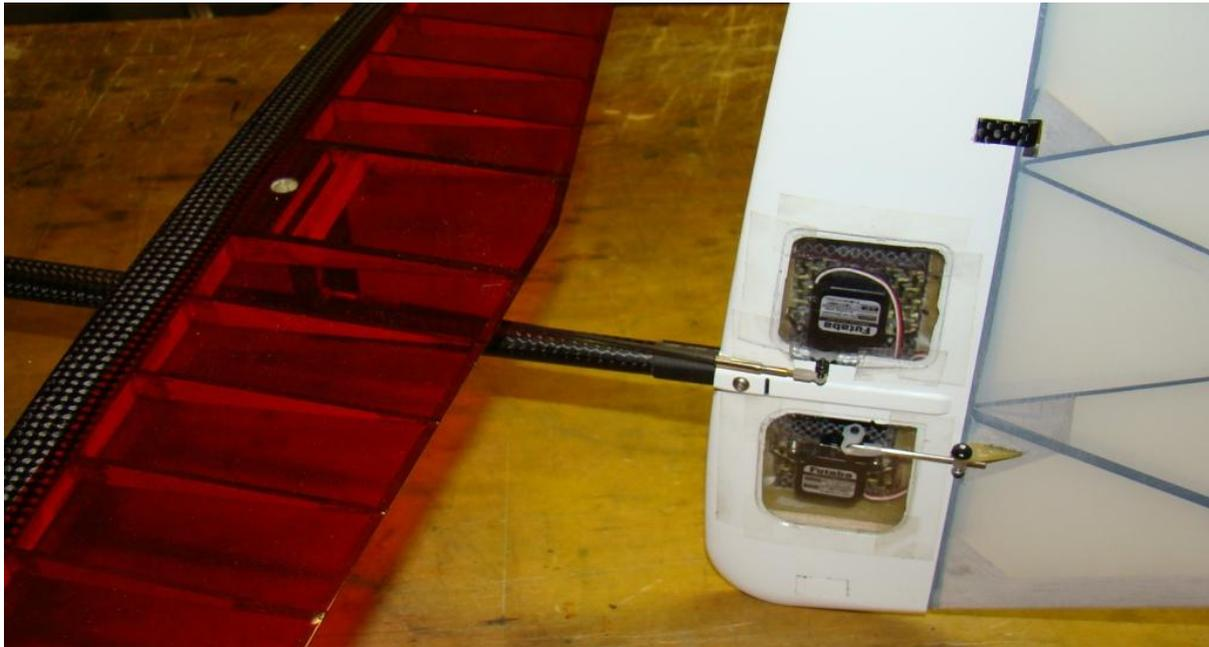
Fig. 4: The rudder and elevator servos are installed in the fixed part of the rudder
