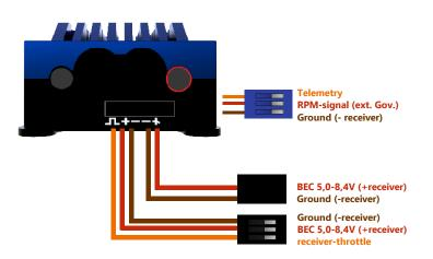
Usually in helicopters, the receiver- and BEC-cables will be wired from the front to the rear alongside the motor. Make sure that the receiver-, tele- and BEC-cables have to be wired together on one side!
