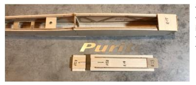
Then glue part R20 centrally on the fuselage planking R22 and fit it together with the canopy in the canopy opening in the fuselage.
