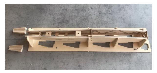
Tip: We screw the fuselage slipway to our building board!
