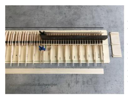
Now the rest of them can too Ribs are aligned. in the They will connect with the Glued spar. After this Step, can also do the Leading edge (CFRP tube 2.5mm) be attached at the front. To note now that the Comb for aligning the Ribs shortened by one field must become. Because now it stands the root rib 5 degrees inclined and thus the comb does not fit more over a full half of the middle part
