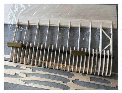
Be careful here: the leading edge in Part A and B are 2.5 mm thick.(In contrast to Part C: here they are only 2mm thick). The wing part B is also again on the leading edge 2mm (under the feet of the Ribs) and on the trailing edge with 8mm underlaid. Thus can the trailing edge free of distortion be glued on. At the end will still be the great reinforcement between the rib B1 and B4 glued in.
