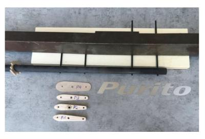
The pylon part P1 can now be fitted and glued in place. For component P2, make sure that the M3 nut points upwards. Attach and glue the P2 and P3 components as well. Only part P4 must not be glued yet, because this will be done later with the elevator. The carbon rods that protrude from the top of the elevator pylon should be shortened to 4.5mm (so that they no longer protrude when the elevator is screwed on)
