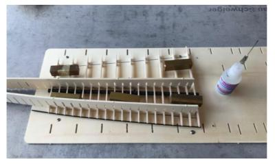
In the end we still check once the correct alignment all ribs and glue all together whole ribs (not the Half ribs) with the pipe. Tip:for correct alignment we use weights to fix the wing part neatly. We use thin one Superglue We use the 2mm CFRP tube as the leading edge, which is carefully inserted into the designatedMilling is inserted. Then the half-ribs can also be used with the comb neatly aligned and glued once
