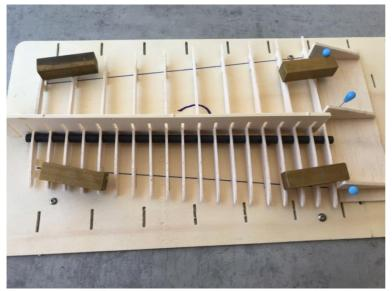
One more note on the Base plate: the foot on the Determines the trailing edge of the rib die Position. Then the ribs can from part C to the cut to length CFRP tube (7mm diameter,262mm length). The CFRP should be at the edge arch Pipe about 7mm survive. The ribs will aligned with the combs.Then you can go to the Template for the feet of the Ribs tucked into part C
