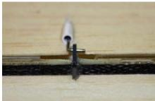
Hold the aileron in zero-position with a ruler. Now put a drop of super glue in the carbon pipe to fix the length of the pushrod.
