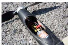
Further electronic equipment (2 servos, receiver) is situated in the rear part of the fuselage.
