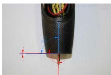
Bend a **steel wire** as shown for **fixing the accumulator** in the fuselage.
