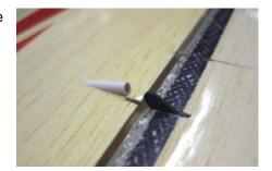
The **hole** in the lever should be a little bit **in front of the turning axis** of the rudder.
