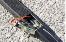
**Suggestion for a servoboard** for the rear part of the fuselage.
