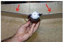
Die **EWD** (angle between wing and elevator) must be **1.8**°. Normally, the angle results automatically, if you mount everything correctly. Nevertheless you should check the angle before you glue everything. Proceed according to the drawing below:
