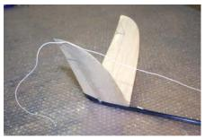
Another possibility is to lay the antenna **inside the gap of the aileron**. For improving reception on **carbon wings** you can solder the antenna to a steel wire, d=0,3mm, which you fix at the end of the wing and let stand out to the back about 10-15cm.
