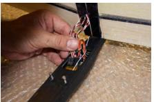
If you have a **hard landing**, always **check** if the engine frame is still fully glued before you make the next start! Also check if all other parts are still working.
