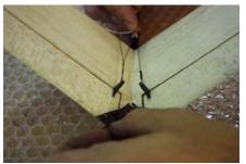
**Drill a small hole in the boom** to lead the wire inside the fuselage to the servo.
