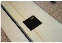
Mill a slit in the root rib, where you can put the cable in.
