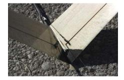
Now, place the V-tail on the boom. Before you glue it, Check the **alignment of the V-tail** regarding the axis of the fuselage and the **EWD**, so that it is fixed correctly.
