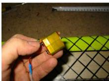
Glue the servo with Stabilit Express or with a 5minute epoxy.
