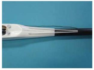
Pushrods outlets: white plastic tubing guides the 0,8 mm carbon rods. The other guides are ca 20 mm long, in ca 15 cm distances, glued on the tube surface.
