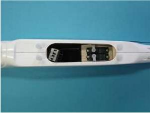
Right hand surface: ESC Castle Phoenix 25. Left hand surface: voltage controller VR3 supplies 6 servos
