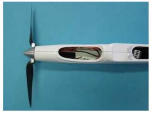
Top view. There is enough space for ESC and voltage regulator (on sides) and battery in between (not shown). The spinner 32 mm provides enough space for the ourunner 28 mm dia with the input cables.
