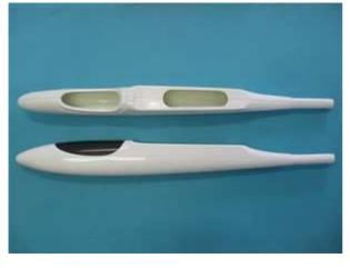
The pod is very sleek. It is long enough to accept 14" dia. Folding prop. The bottom part is flattened to obtain more space for the equipment.
