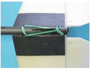
Secure the V-tail with rubber band. Simple and effective.
