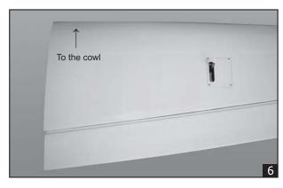
6. Repeat step # 2 - # 5 to install the second aileron servo in the opposite wing half.
