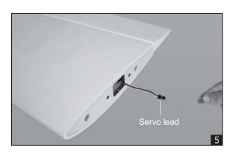
5. Place the aileron servo tray / hatch into the servo box on the bottom of the wing and drill 1,6mm pilot holes through the tray and the servo box for each of the four mounting screws. Secure the servo tray in place using the mounting screws provided (2mm x 12mm).
