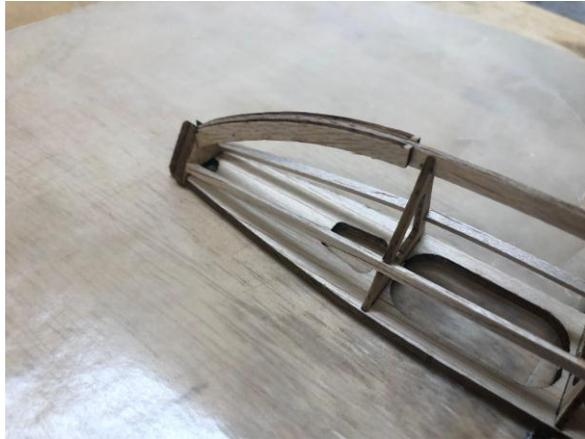
7. You can now un-pin the fuselage from your table and locate formers F-3, F-4, F-5 and F-6. F-6 is not marked due to its size. Install the remaining magnet flush with the front of F-3 using Med CA. Glue formers in place again being sure to keep them 90 degrees to the crutch.
