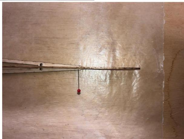
5. Locate 2 of the  $\frac{3}{32}$ " stringers. These are taped to the inside of your kit box along with the pushrods. These will need to be trimmed to the proper length before being glued in place. Note that the front bends to meet the rear of N-1, and also sits a bit proud at the rear where it joins F-5b. This will be sanded flush later.
