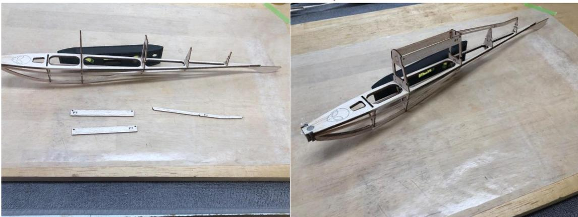
9. Locate the two shorter  $\frac{3}{32}$  stringer pieces. These will fill in the area behind the wing saddles back the spine and F-5. These will also be trimmed to fit, glue in place.
