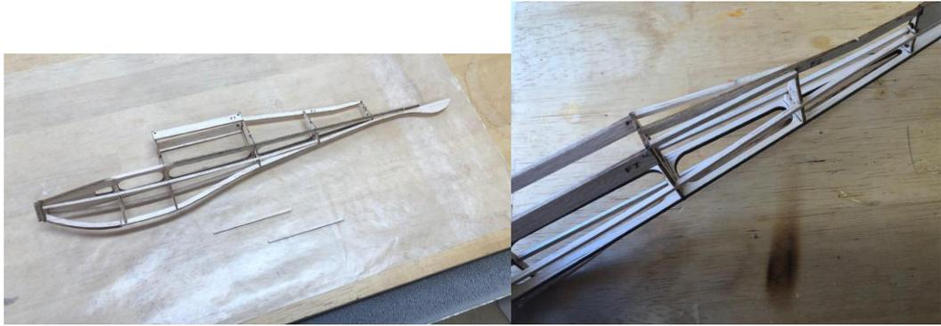
10. Locate the  $\frac{1}{32}$ " tail saddle pieces. Glue these one at a time to the crutch and F-6. Again make sure that these are square and vertical. A small gap remains at the top front area for the fin to slide between.
