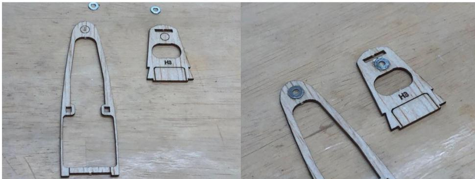
13. Glue H-3 (facing aft) to H-1 keeping it square. Fit H-2 in place (1/8") and glue. Glue H-5 into the slot in H-3, again keeping it square.
