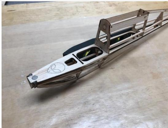
12. Locate H-1 (hatch base), H-3 former and two washers out of the hardware bag. Remove the area inside the etched circle with the tip of an X-acto blade until the washers sit flush with the surface. When satisfied glue in place with Med CA.
