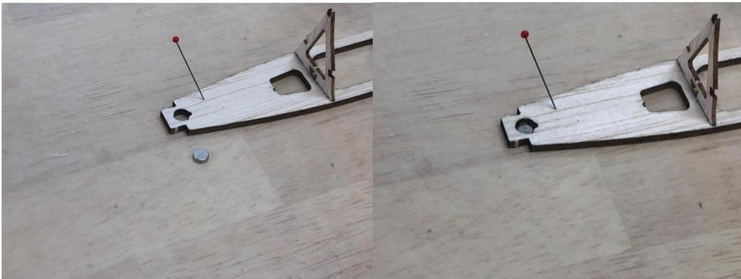
3. Locate the N-1 & N-2 nose blocks. Glue N-1 in place first followed by N-2. Try to keep glue away from the edges, this will make sanding later much easier.
