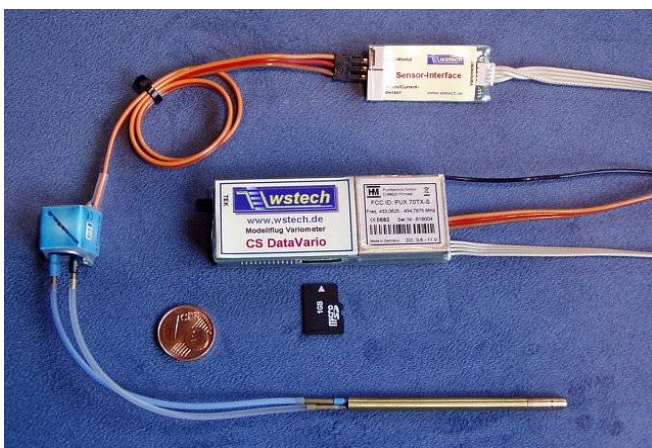
CS DataVario with Sensor Interface a. Speed Sensor
