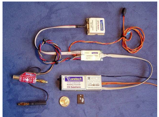
With Sensor Interface, GPS, Current- a. Temp. Sensor
