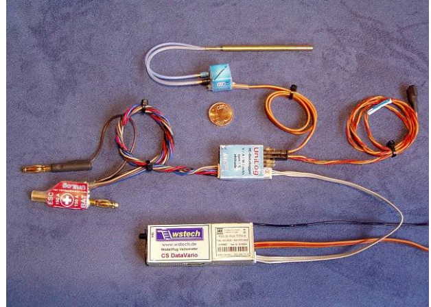
here with UniLog a. Current, Speed- a. Temp. Sensor
