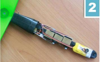
3) Glue servos with CA, but leave the battery mounted with tape.
