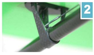
3) Put the stabilizer/V-mount back on the tail boom and align it with the wing. Glue the V-mount with thin CA.
