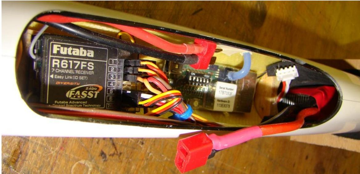
Fig. 9: Layout of elements in the front of the fuselage. The front of the plane is on the left.
