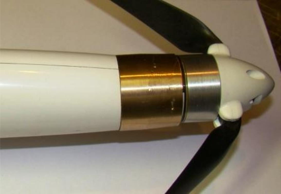
Fig. 6: Propulsion system: the motor is attached in front of the fuselage, rather than installed inside. The brass adaptor is fixed and surrounds the motor. The aluminum adaptor rotates with the propeller.
