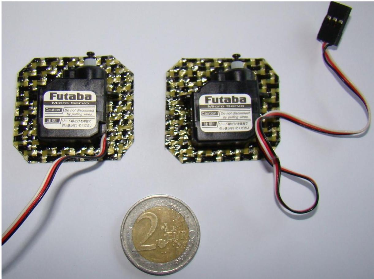
Fig3: Futaba S4114 servos glued to a piece of carbon-kevlar-epoxy composite and blocked by the epoxy
