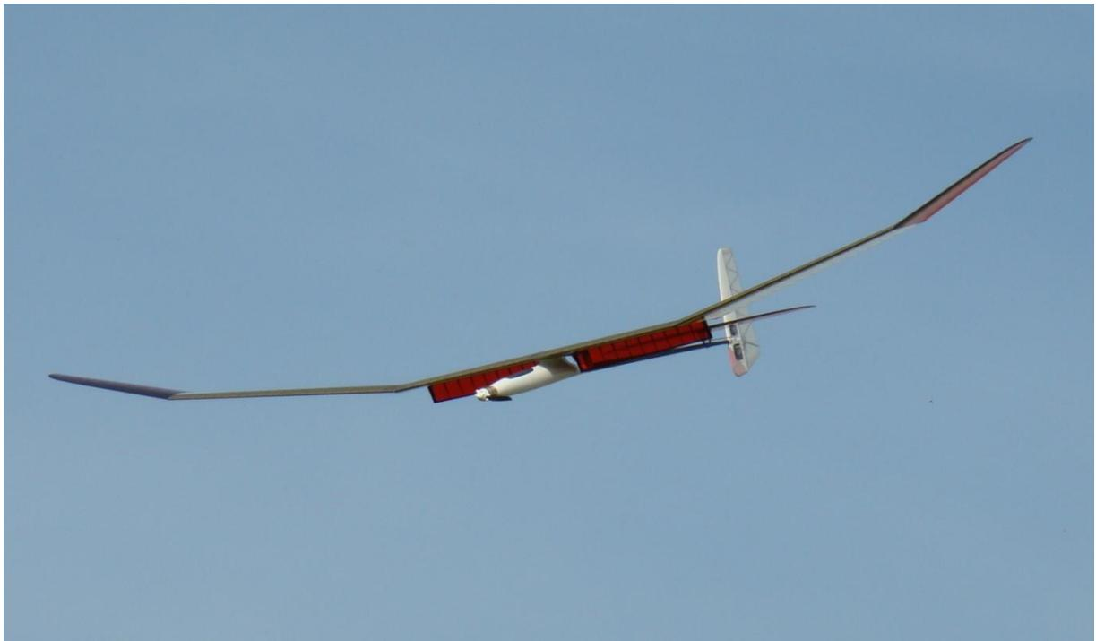
Fig 15: The AVA Pro-e in a steep but slow dive with the flaps down
