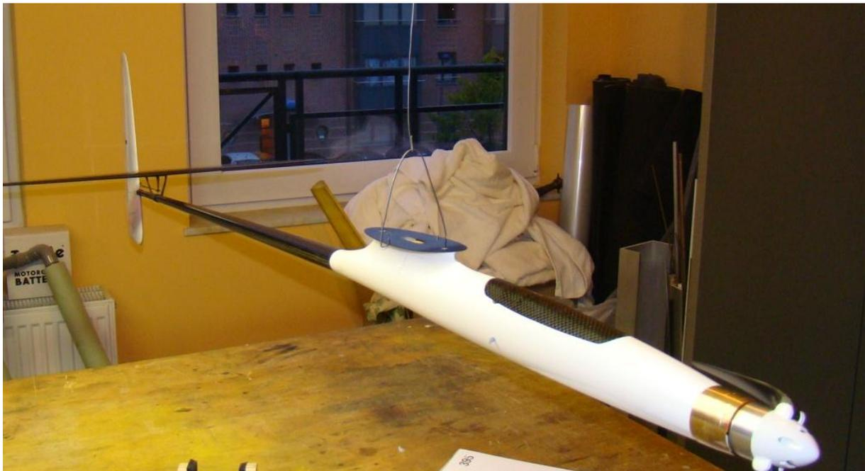
Fig.8: Suspension jig used to balance weights in the fuselage
