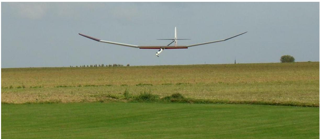
Fig. 15: The AVA approaching landing with the flaps down. It's time to put the flaps back up to avoid damage when the flaps hit the ground
