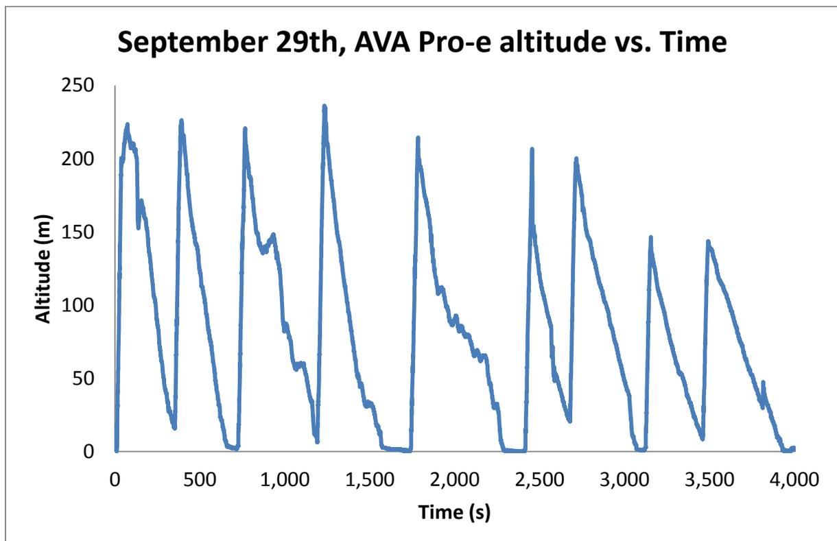
The first observation is that I could fly a quite long time (more than one hour) on a single battery, a 3 elements Li-Po of 2200 mAh capacity. As can be seen, I could climb 9 times out of this single battery. In climb, the motor uses around 25 Amp. so the time to discharge the battery is around 5 minutes, or 300 seconds.
