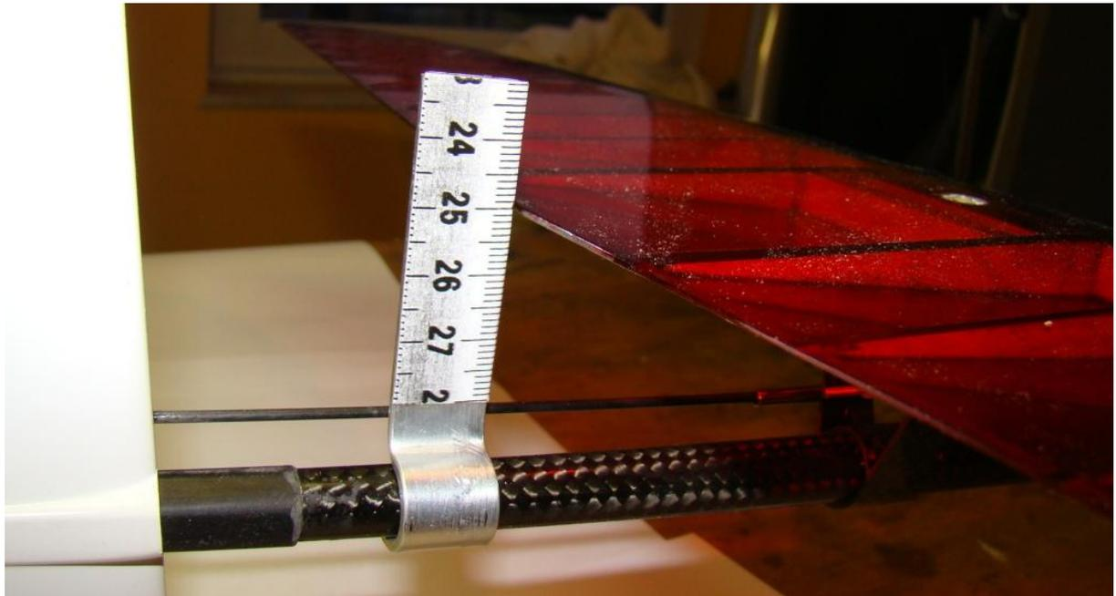
Fig. 11: Small tool to check the elevator settings
