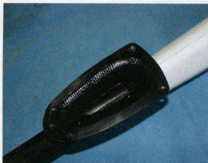
Pylon wing mount is part of fuselage pod and tail boom is ready fitted
