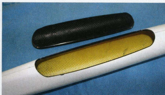
Fin and AMT mounting is in carbon fibre and ready fitted to the tail boom
