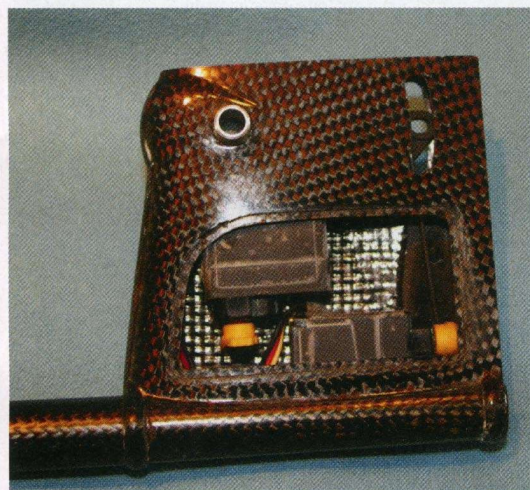
LEFT: Servos eventually slotted into tail servo cover!
