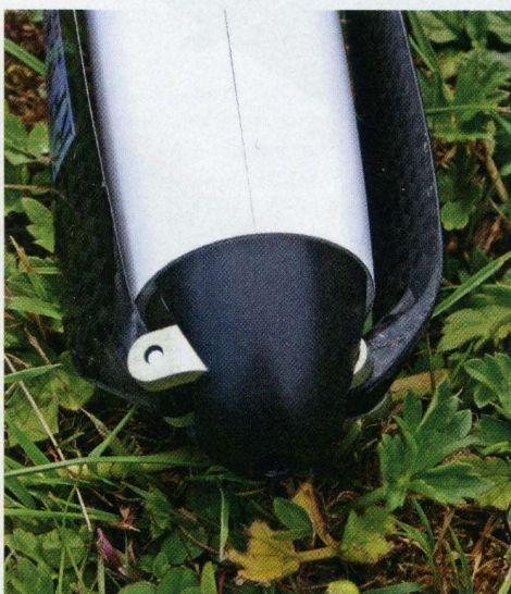
ABOVE: Twisted yoke keeps propeller flat to fuselage minimising drag
