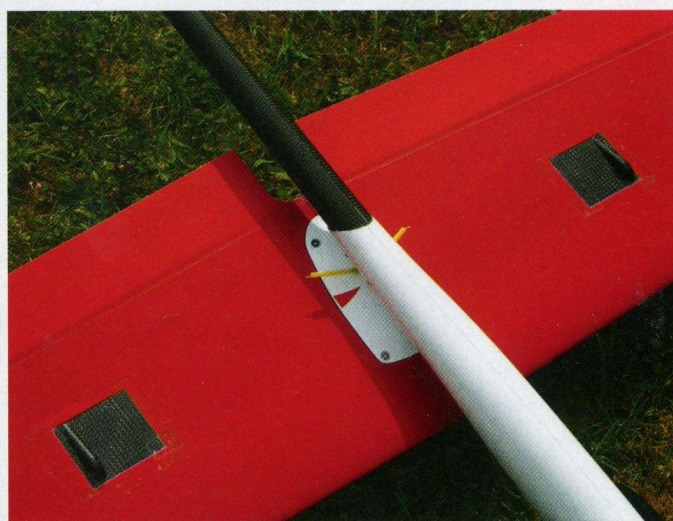
ABOVE: Wing secured from under pylon. The two yellow tubes protect Futaba 2.4 GHz aerials and maintain correct orientation
