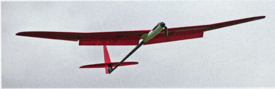
With flaps deployed, the model could be slowed safely to a walking pace, whilst retaining full control
