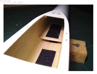
battery is moved for fine tuning the balance point. I had no problems in achieving the correct C of G and marked the appropriate battery positions inside the fuselage with a marker pen for easy visual future reference. The battery and receiver trays were then permanently installed with epoxy and micro balloons, allowing enough length in the battery tray to provide sufficient movement of the battery for adjustment in flight tests.
