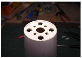
trial fitting the motor and gearbox. I also marked and drilled four 6mm diameter cooling air holes in the bulkhead as the nose section as supplied has no factory cut cooling air holes.
