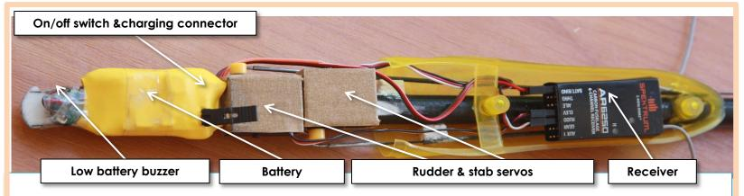
Place RC as above. Centre the output arms & glue servos in place. Trim the pushrods to length, thread on 2cm heat shrink tubing. Test fit and then CA the Z bend wires to the pushrods. Slip on the heatshrink tubing and heat to secure joint. Add more CA. Remove servo arms and thread onto Z bends. Tape the battery in place.
