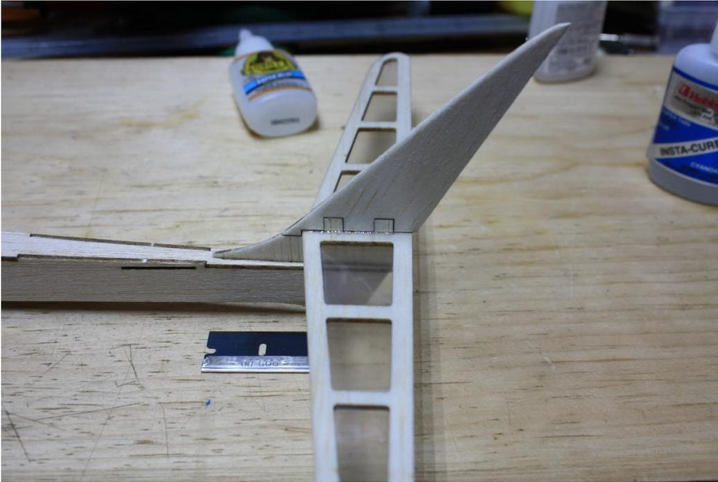
Glue the control horns into the surfaces. Pay attention to what side they are on, keeping in mind what side each slot is on. Here, you are looking at the bottom of the elevator, and the right hand side of the rudder.
