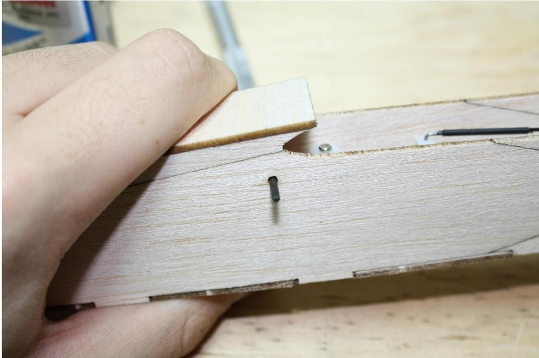
Now bend up the highstart hook, and tack glue it to the 1/32" plywood plate (it only goes in in one direction). The drawing for the hook will be on the last page of the pages of paper included with your kit.
