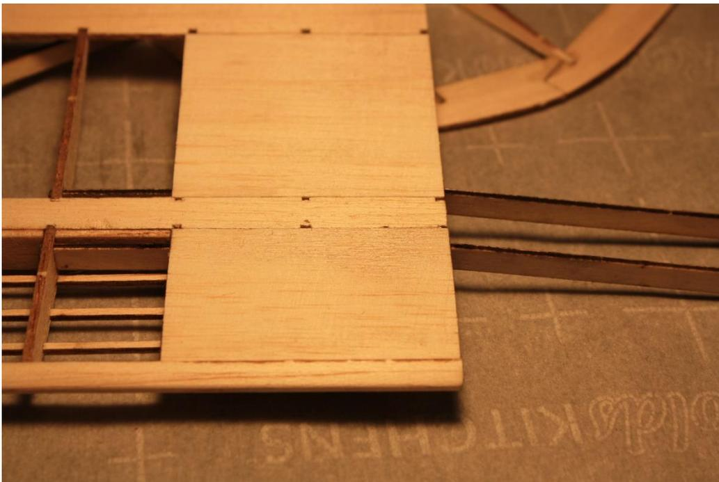
Now, slide the other wing half onto the joiners, and slide it almost all of the way together. Slather one rib in ca, and put some on the joiners close to where they enter the rib hole. Then, slide the wing together, and glue the joiners where they go through the other ribs.
