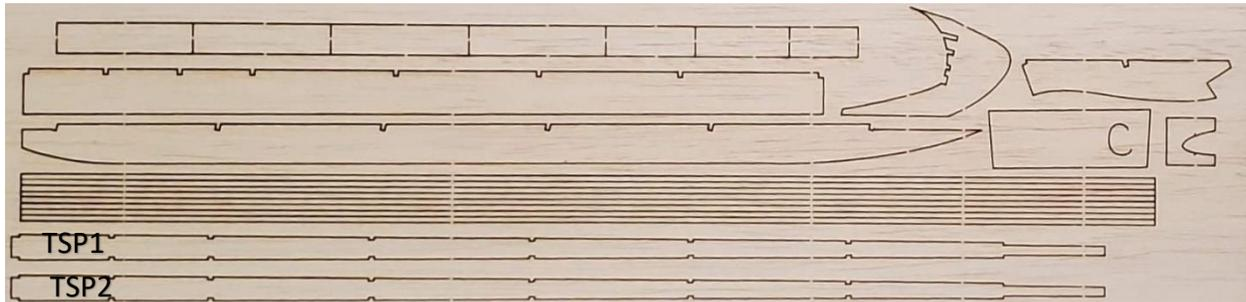
You'll need a few sheets of wood for the wing. You'll need the sheet of 3/32" balsa, the sheets of ribs (1/16"), the sheet of 1/32" balsa, and the sheet with trailing edges, turbulator spars, shear webs, angle gauges, and a few other things (1/16" thick).
