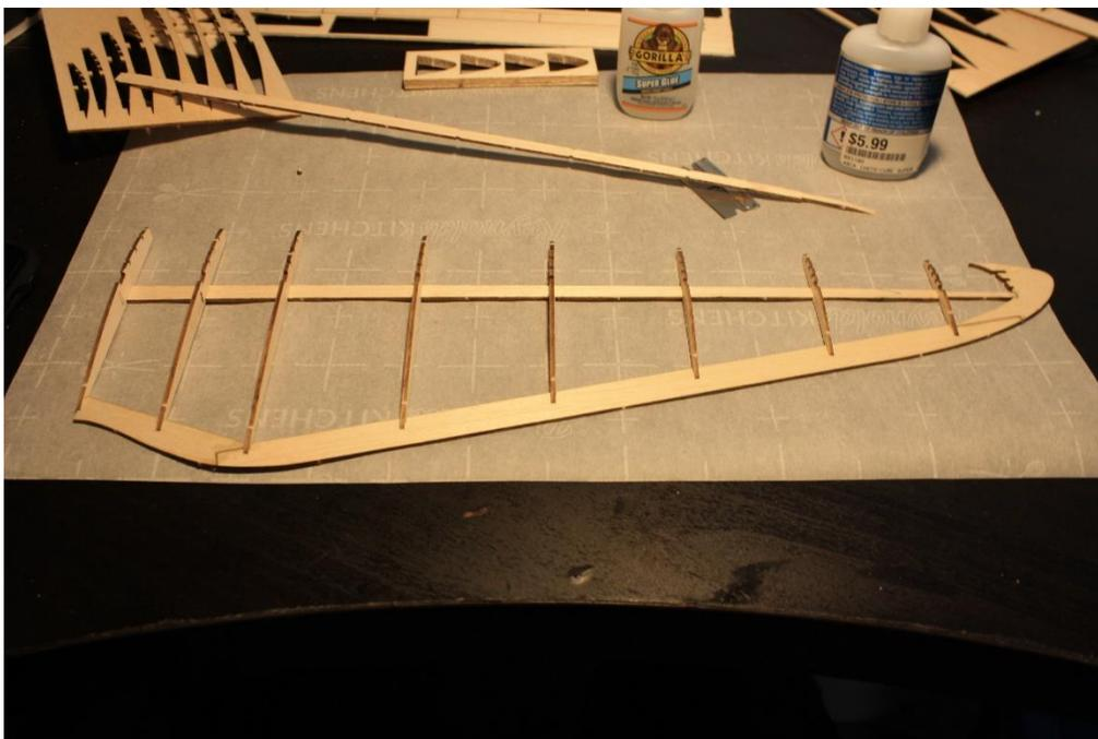
Get the top wing spar (TSP2), and round off the bottom of the tip as shown, then, slot the spar into place.
