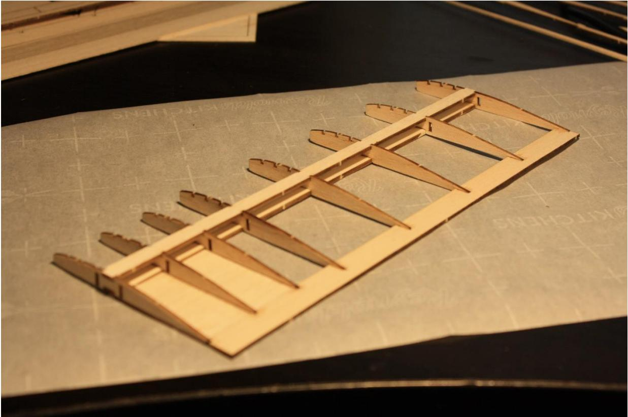
Moving on to the outer wing panel, assemble the trailing edge as shown
