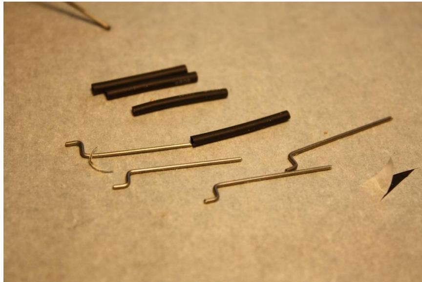
Grab the carbon rod and a lighter/soldering iron/ heatgun, and slide a piece of heatshrink over the carbon, then, insert a Z bend, and shrink the heatshrink. Once it's cooled off, grab and twist the z bend out, and slide the piece of newly molded heatshrink off. Repeat this another 3 times.
