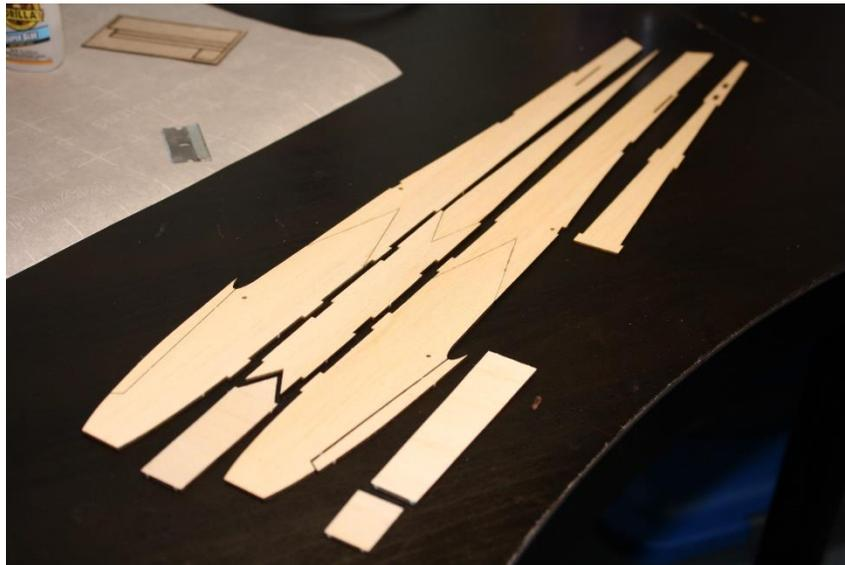
This stuff will come from 2 sheets. One sheet with most of the stuff, and then a tiny sheet with the crossgrain balsa. Locate those sheets, and you'll be good. Grab the piece of crossgrain balsa with the triangle on the end. This gets glued onto the bottom sheet as shown.
