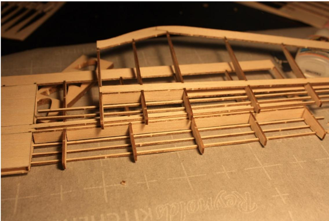
Go back to the inner wing panel, and glue the 3<sup>rd</sup> longest (S2) piece of 1/32" balsa to the bottom of the 3 ribs, and to the main spar.
