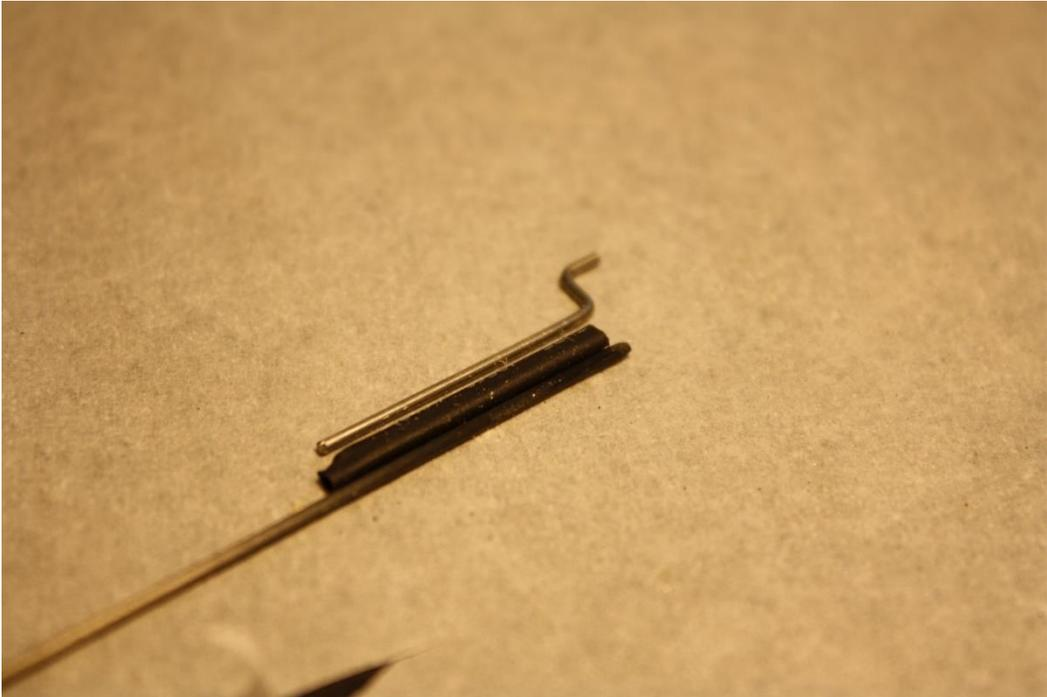
Slide a piece of carbon rod into the elevator slot, stopping it just short of the elevator servo horn. Now, cut it just short of the control horn. If you took the carbon rod out of the fuse, re-insert it. Slide the heatshrink tube over the carbon, insert the Z Bend into the elevator horn, and then slide the heatshrink over the z bend. Hopefully the pictures demonstrate this, it's not the easiest thing to explain!
