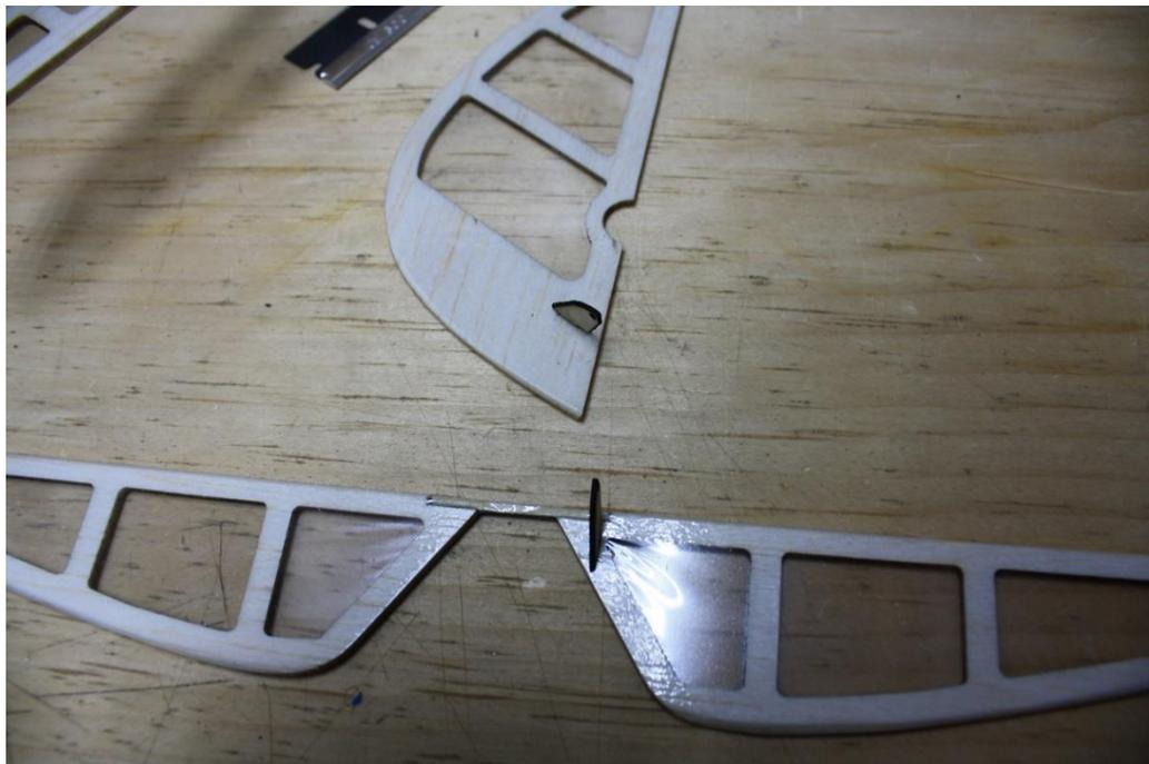
Get some hinge tape, and put it on the elevator. Cut the tape to size, and trim off the excess that's around the joiner and such. Also, cut a slot to clear the vertical stab.
