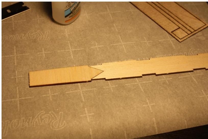
Next, glue a side onto the fuselage bottom. Make sure you get the sides correct. The one with the high slot in the rear goes on the left, the side with the lower slot goes on the right. Just glue the straight center section in place for now. Don't glue the front and back sections in place.
