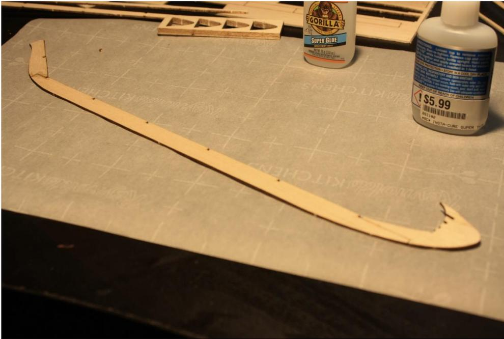
Grab your 1/16" wing spars. Like before, there is a top and bottom wing spar(TSP1&TSP2). The top spar is the one with the longest slot at the wide end. Get the bottom spar(TSP1), and glue it into the farthest aft slot in the wingtip. Grab your wing rib sheet, and dry fit all of the wing ribs (9-16). Rib 9 at the root, rib 16 at the tip.
