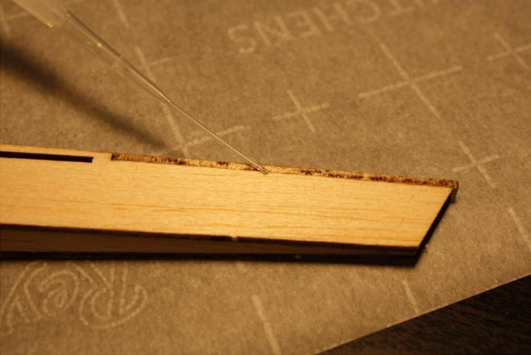
Go back to the front of the fuselage. On that crossgrain parts sheet, grab shortest piece of wood. Glue it to the top of the fuselage on the front. Sand the front of the fuselage flat. Grab the 3/16" sheet, stack the noseblocks up, and glue them to the front of the fuselage. Your noseblock will fit a little better.
