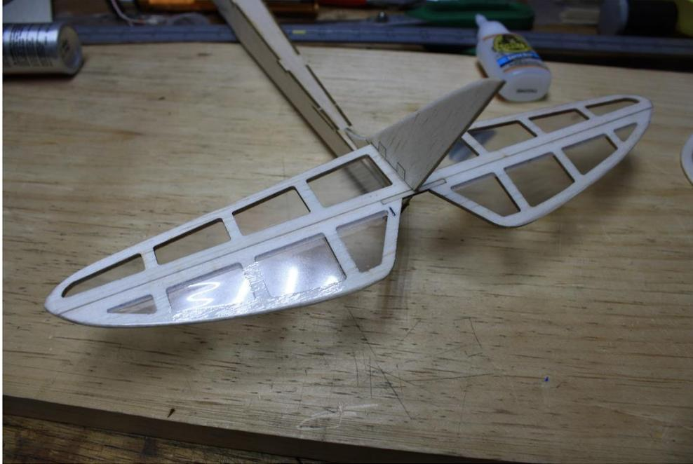
Do the same on the rudder. Once it's on, put hinge tape on the skid, as well as the sub fin, not just the top vertical stab portion.
