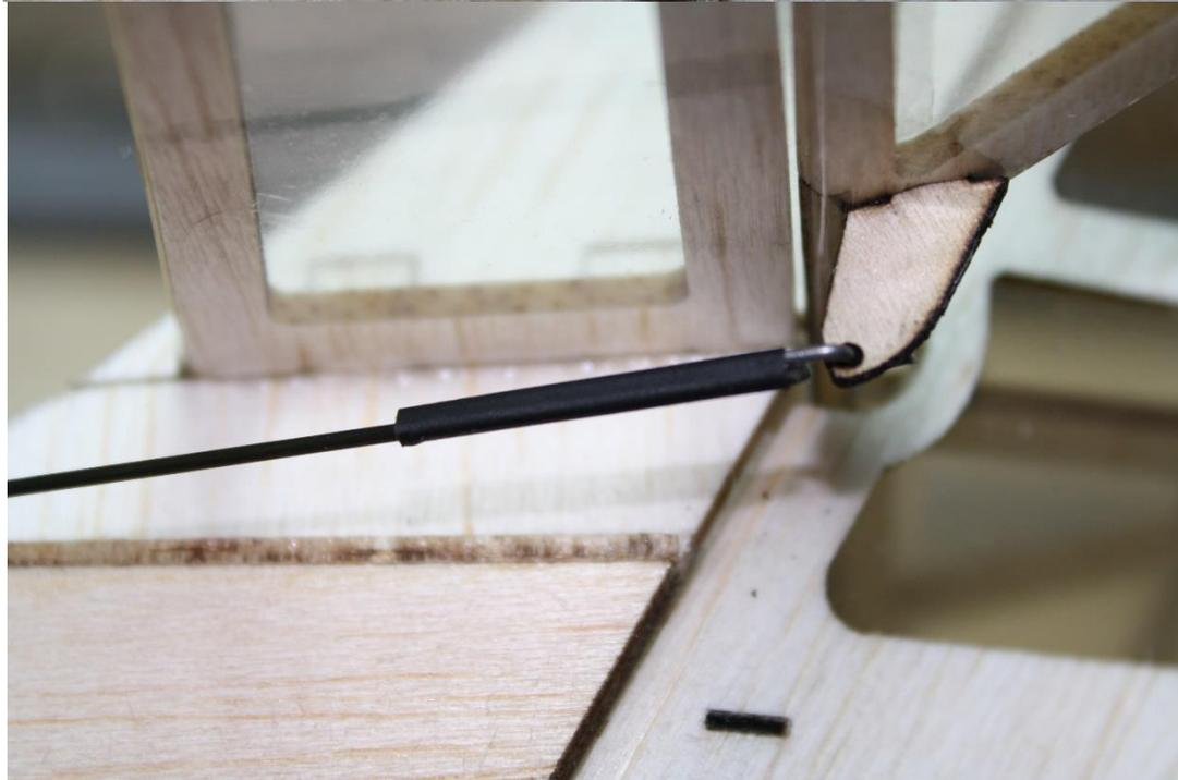
This rod will go to the front servo, so cut the carbon rod about 1/8" short of hitting the servo center.
