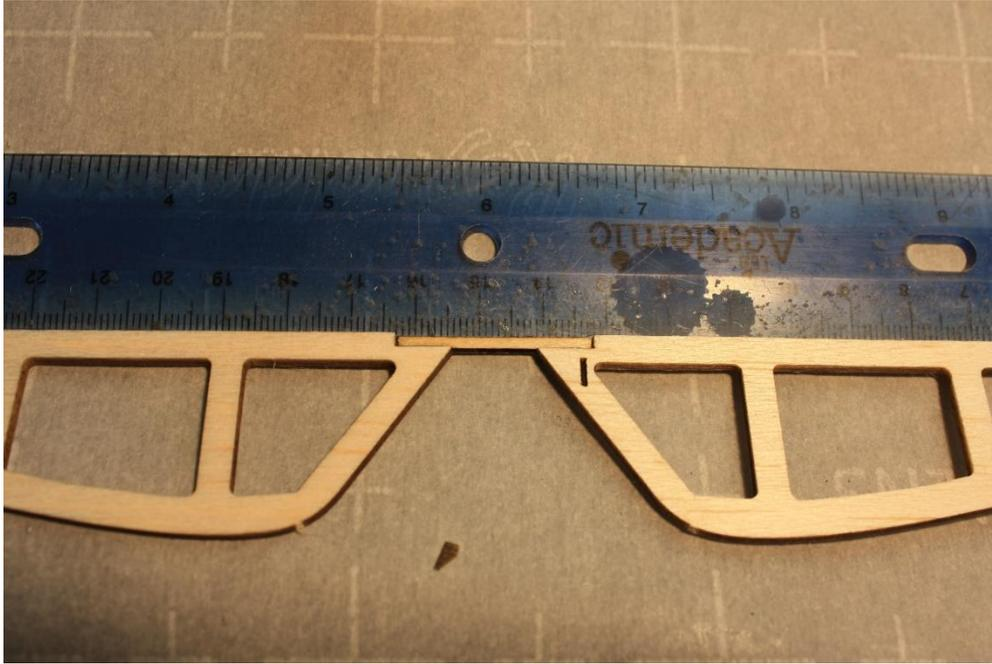
Bevel the bottom of the elevator. You will have to slightly sand a bevel into the joiner. On the rudder, you will have to bevel the left hand side of the rudder, as the control horn is on the right. Now things are beveled, round off all of the edges. Rudder, elevator, horizontal stabilizer, vertical stabilizer, the underpart of the vertical stabilizer, and the skid on the fuselage.
