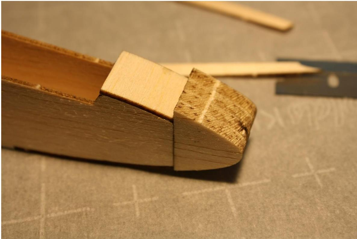
Grab the longest crossgrain piece of balsa, the little canopy rails from the fuselage, and your sheet of 1/64" ply. Assemble as shown.
