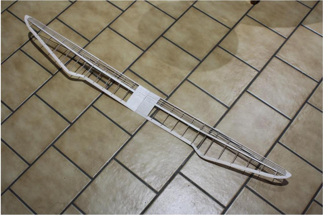
A quick note to mention **before** you start the tail surfaces. In this kit, we are including two rudders. The smaller one is the direct scale down, and the fatter one is one we drew up; to increase turning authority.
