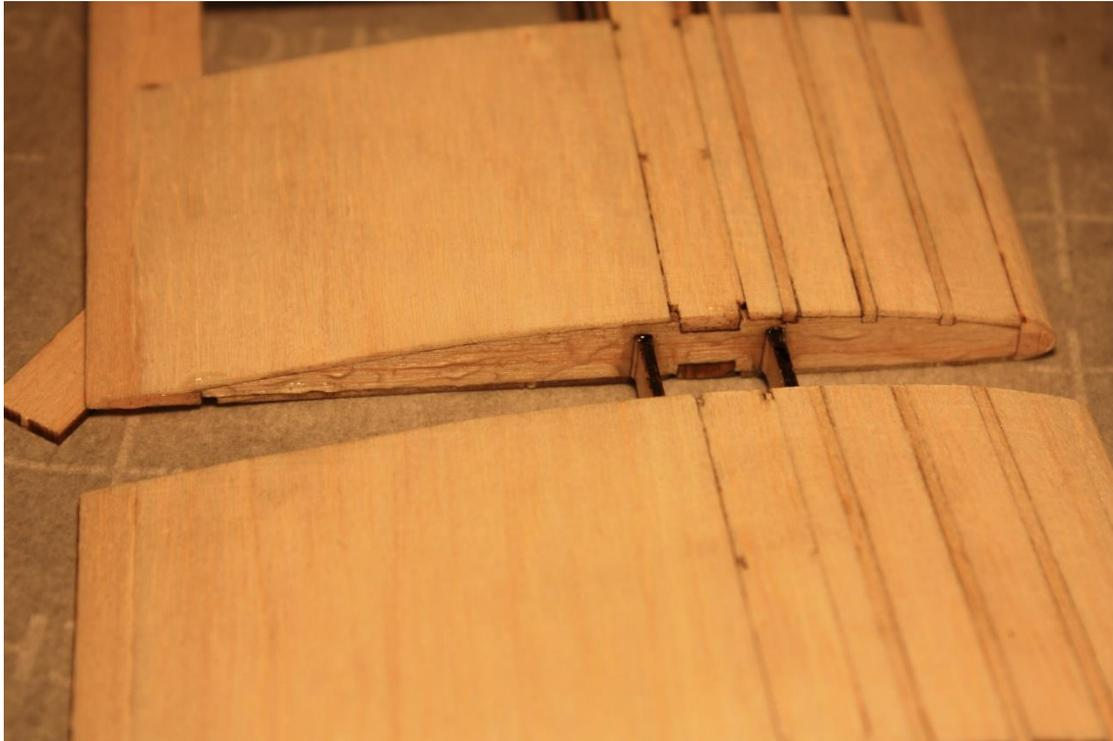
To really tie it all together, rub ca into all of the spar joints. This will make the wing substantially stronger.
