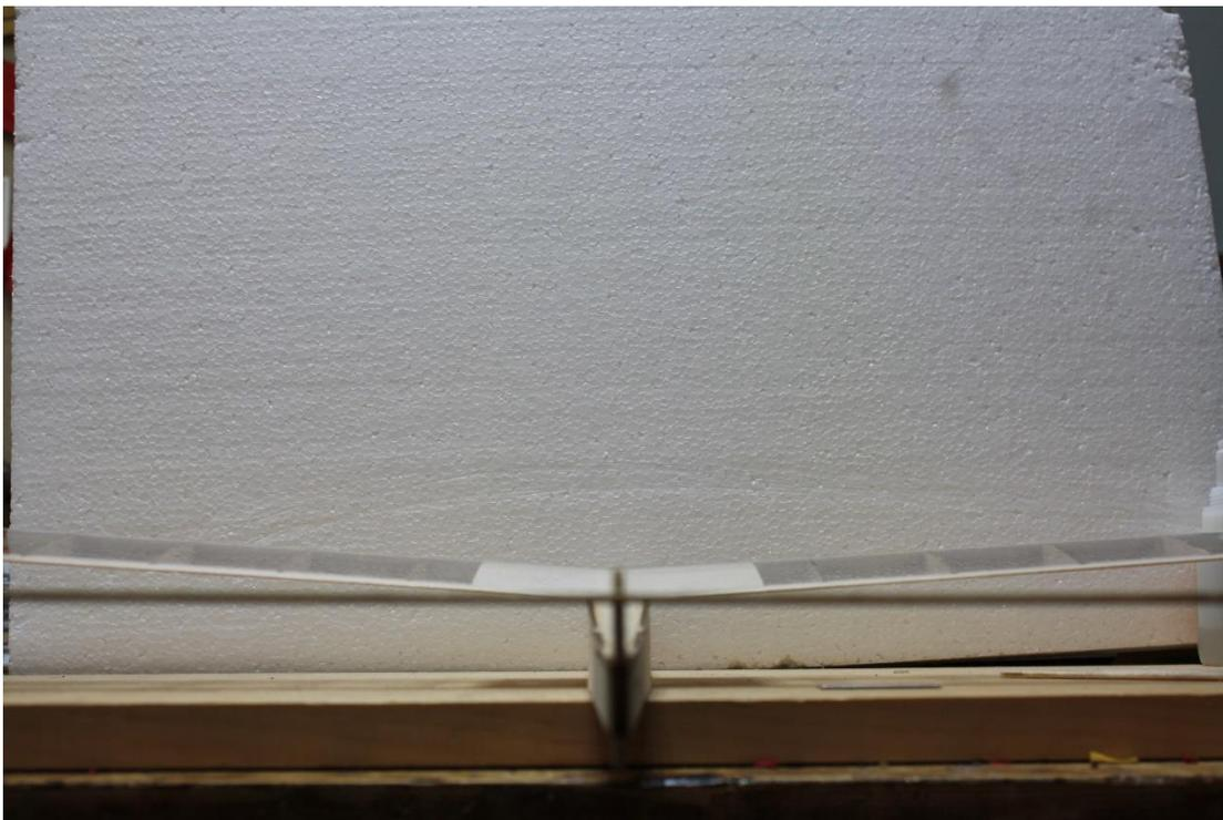
Put the rudder on the sub fin, get it 90 degrees to the horizontal stab, and glue it in place too.
