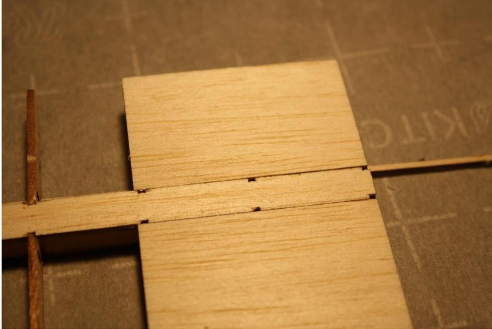
Grab the 1/16" sticks from the parts sheet, and glue them into the slots on the inner panel. Note that the 3 ribs on top of the sheeting have half depth slots, so the stick won't sink all of the way into the rib. Do not force them into the rib.
