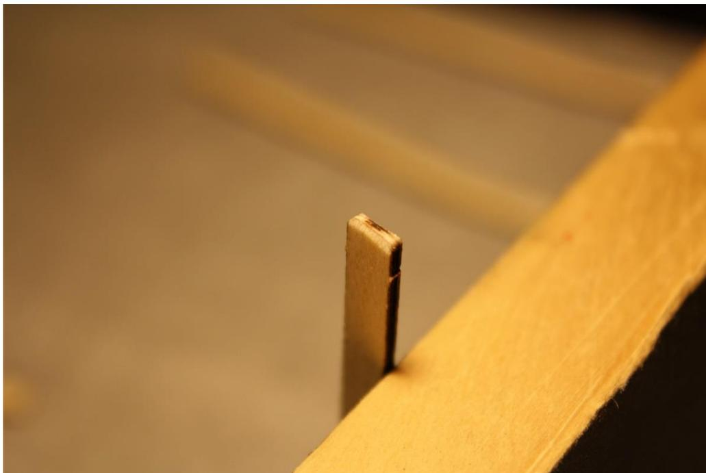
Slide a joiner into an outer wing panel. Glue in place with ca.
