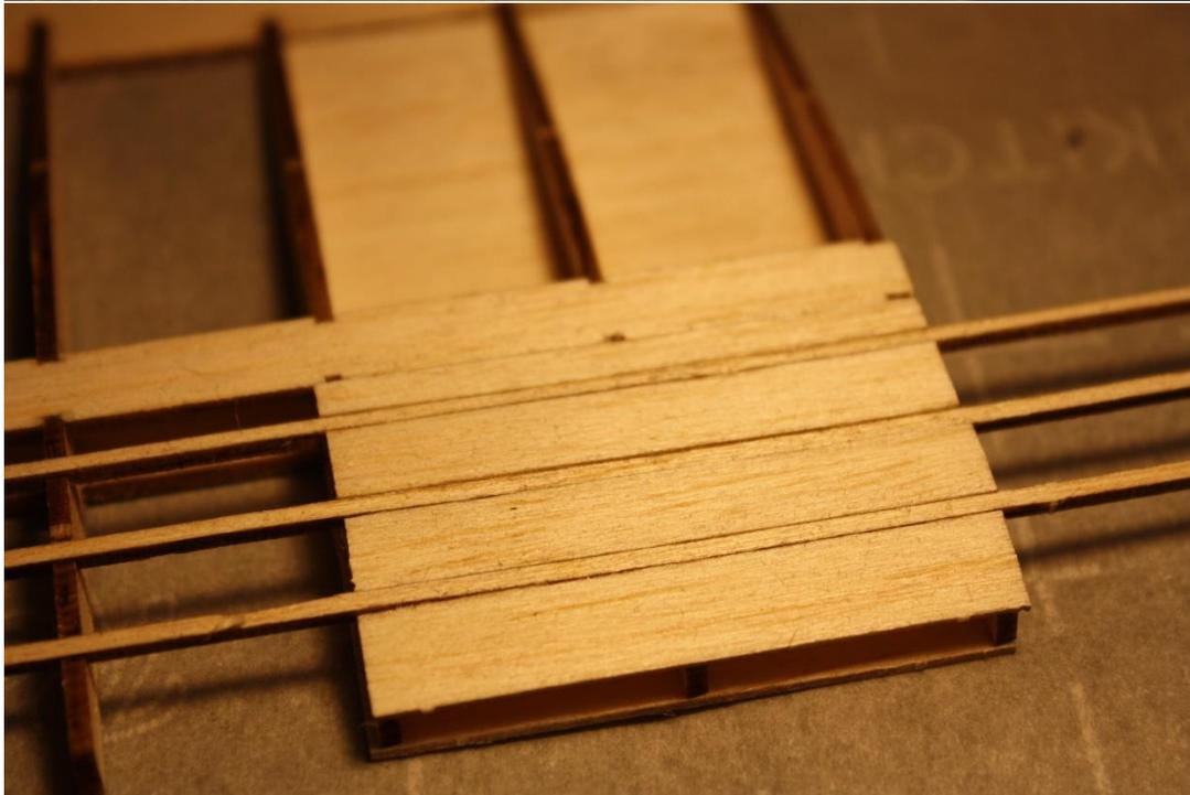
Take the longest piece of 1/32" sheeting (S3), sand a taper into the short edge as shown. Then, glue it onto the 3 ribs, main spar, and trailing edge. I find it easiest to apply glue in all locations, then butt it against the spar and roll the wood onto the ribs towards the trailing edge.
