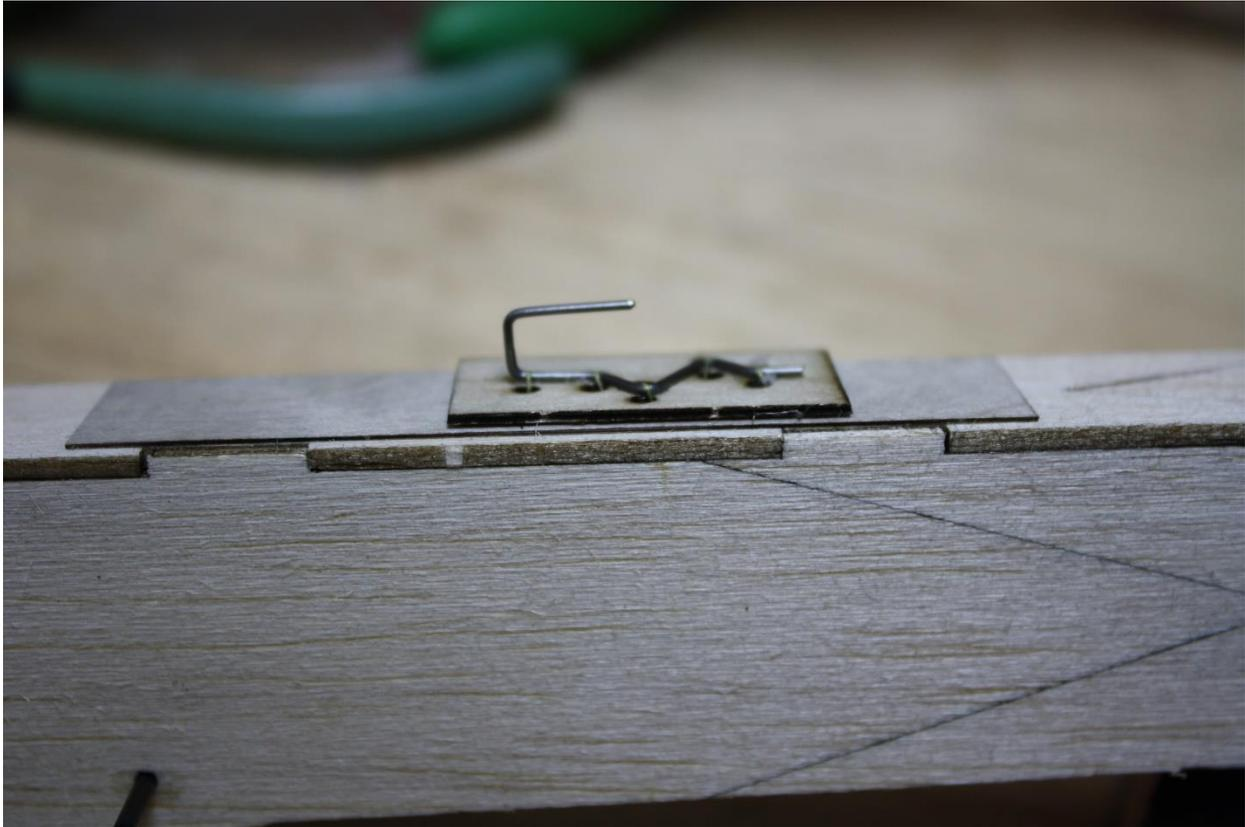
You have a few options to hold the canopy on. If you covered the fuselage, tape is a good option, as it won't lose its stickiness. I prefer to use a rubber band for simplicity. You can hook it over the wing mounting pegs, or just slide the rubber band over the fuselage.
