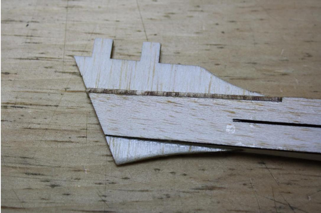
Take the sub fin, and glue it into the fuselage, taking care to keep it vertical. Do the same for the skid, keeping it flush with the rear of the fuse and vertical too.
