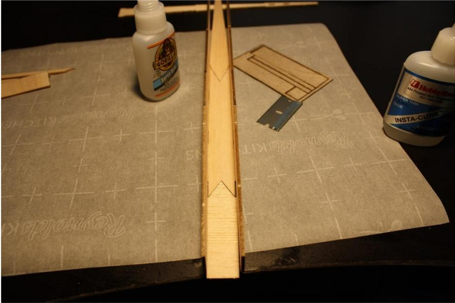
Now pull the sides together in the front of the fuselage, and glue in place.
