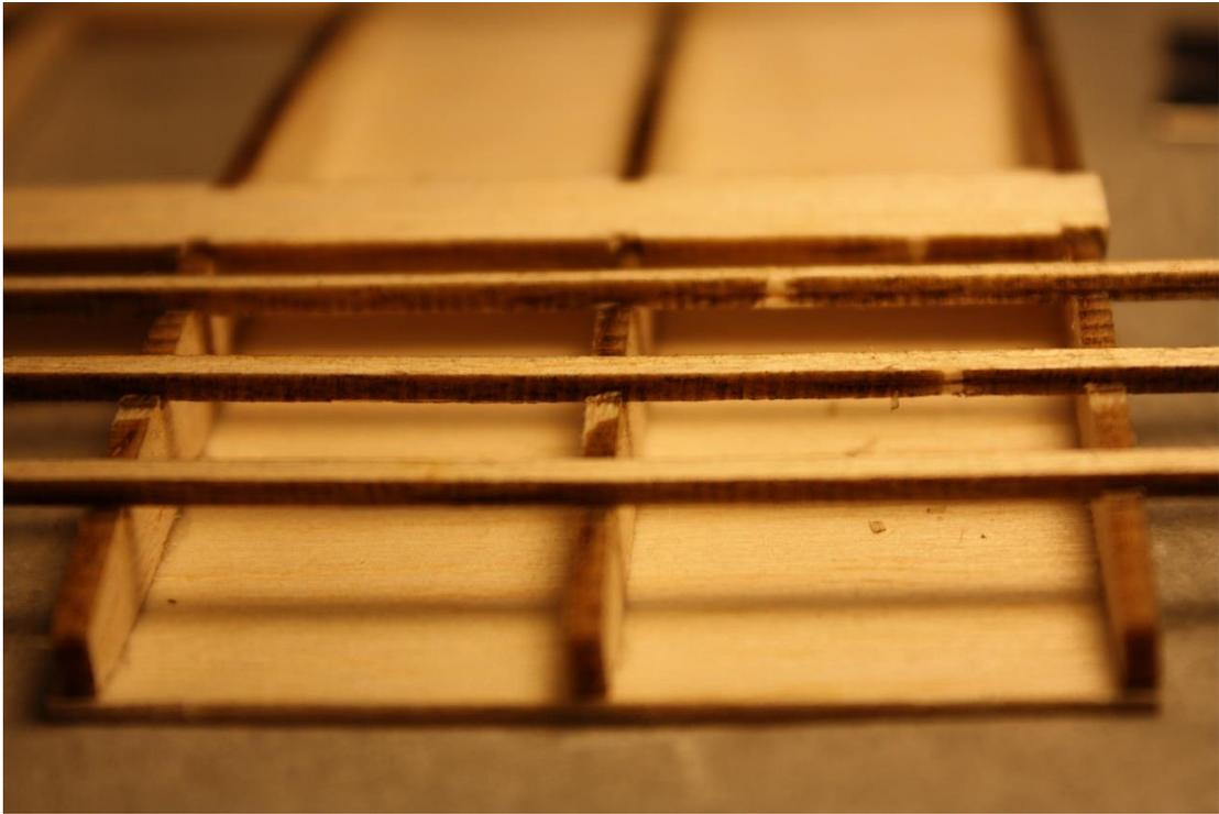
Grab the rest of your 1/32" balsa sheet. Get the 4 small narrow bits of wood (S4-S7). These fill in the slots between each turbulator spar. They are sized to be an almost perfect fit, but you will need to sand them slightly to fit. Just take your time and sneak up on it. Once they are all in, sand the front pieces of wood back to the leading edges of the ribs. This will prep that area for gluing on the leading edges.
