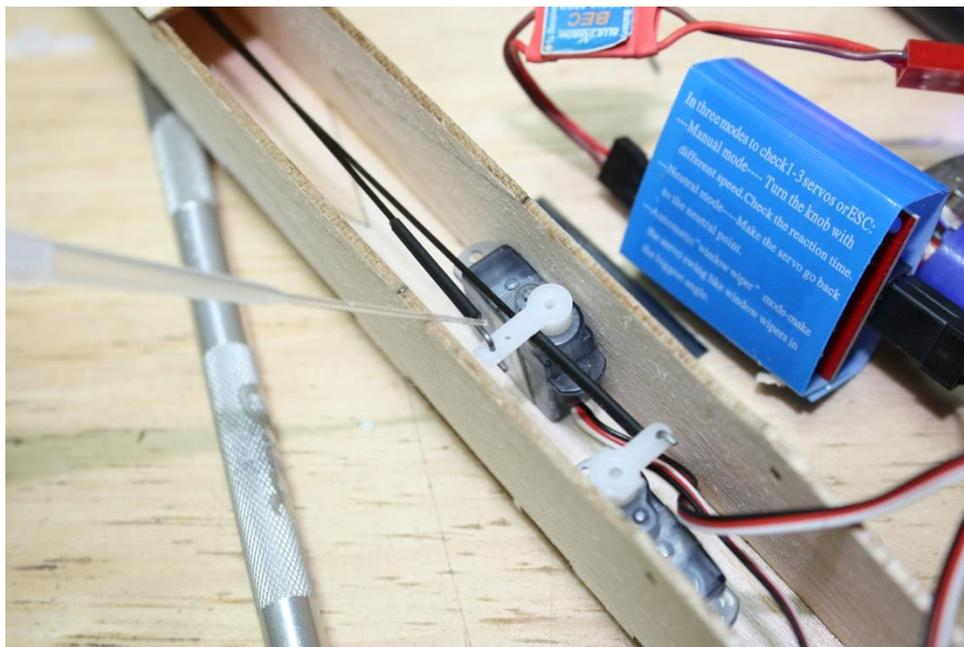
Power on the servos, and center them. Slide the carbon underneath the heatshrink at either end to center the surfaces. Once centered, apply a drop of thin CA to wick into the heatshrink on the servo end as well as the control horn end.
