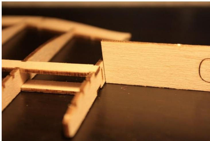
Go out to the wingtip and glue the top spar to the top of the bottom spar as shown.
