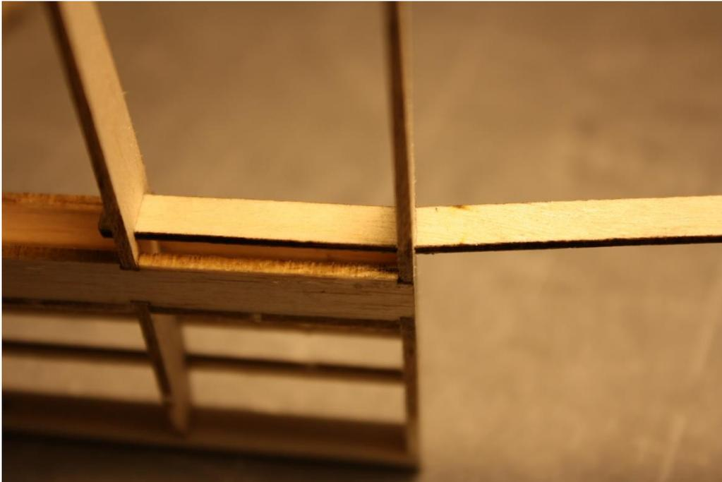
Slide the joiner into the other side of the wing, slather a rib in ca, and glue the outer panel to the center panel. Then apply ca to the joiner where it slides into the rib. I forgot to take pictures of this step, but continue on, the process is identical to gluing the two inner panels together.
